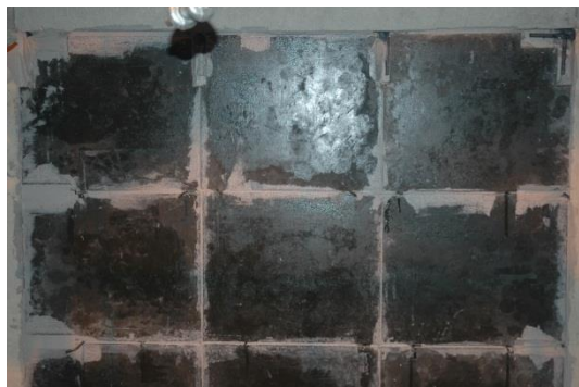
Figure 3.25 Assemblage of ECC Panels on test Frame
