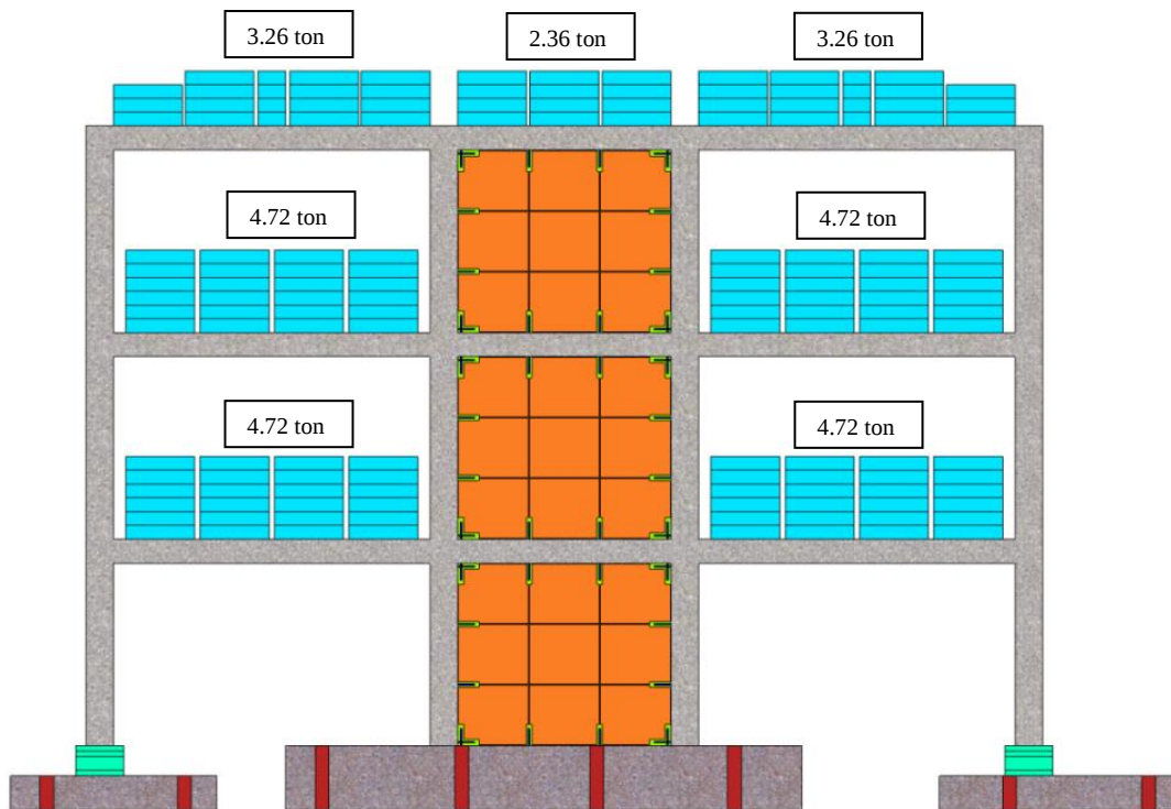
Figure 3.23 General view of strengthened frame
