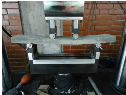
Figure 2.3 Bending test of 510×75×25 mm specimens
