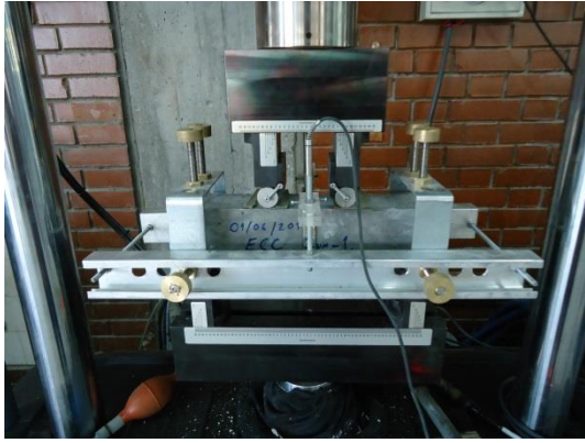
Figure 2.2 Bending test of 315×75×75 mm specimens
