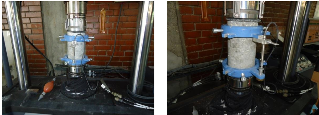
Figure 2.1 Uniaxial compressive test with elastic modulus apparatus
