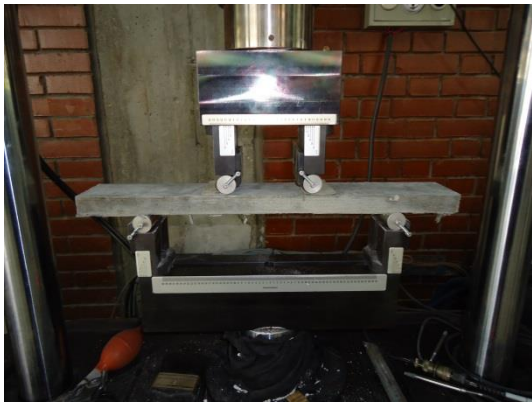
Figure 2.3 Bending test of 510×75×25 mm specimens
