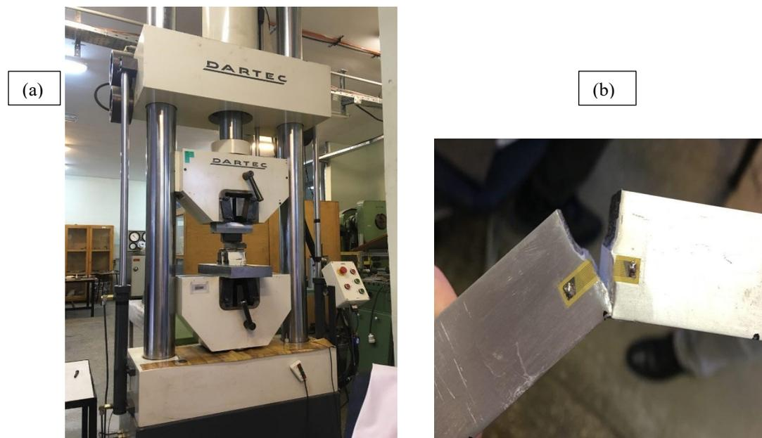
Figure 4. 2 (a): DARTEC machine, (b): Fractured specimen
