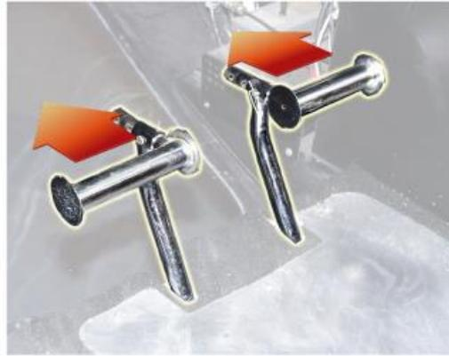
Figure 1-4 Tail Rotor Pedals [5]
