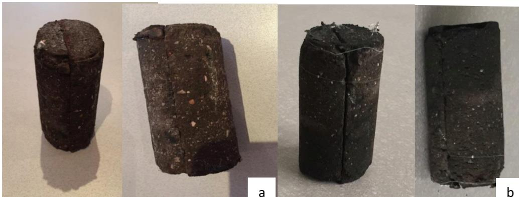
**Figure 7.8** After the Polymer Gel Injection Experiment, Artificially Fractured
