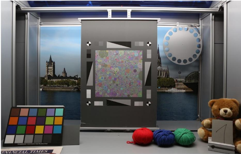
Figure 6.11: The Test Setup Proposed by Image-Engineering GmbH [42]
