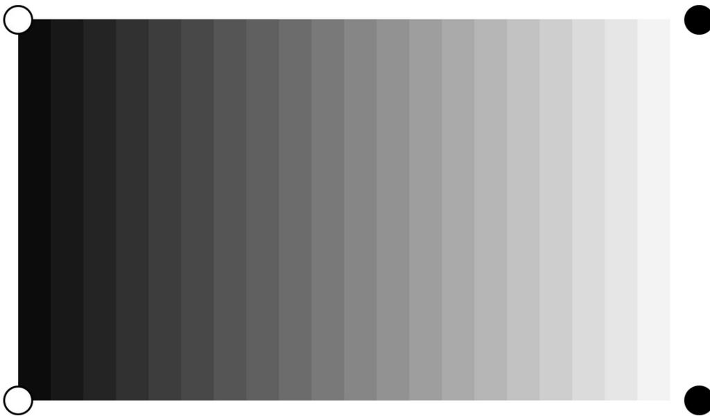
Figure 2.6: The Test Chart for the Dynamic Range Tests
