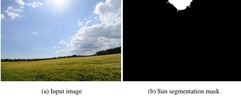
Figure 3.7: Sun segmentation mask in the second image is calculated with a flood fill algorithm from the first image and the user click on the sun. Image taken from [1].
