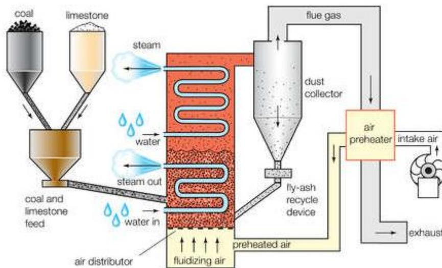
Figure 45 Fluidized Bed Combustion [72]
