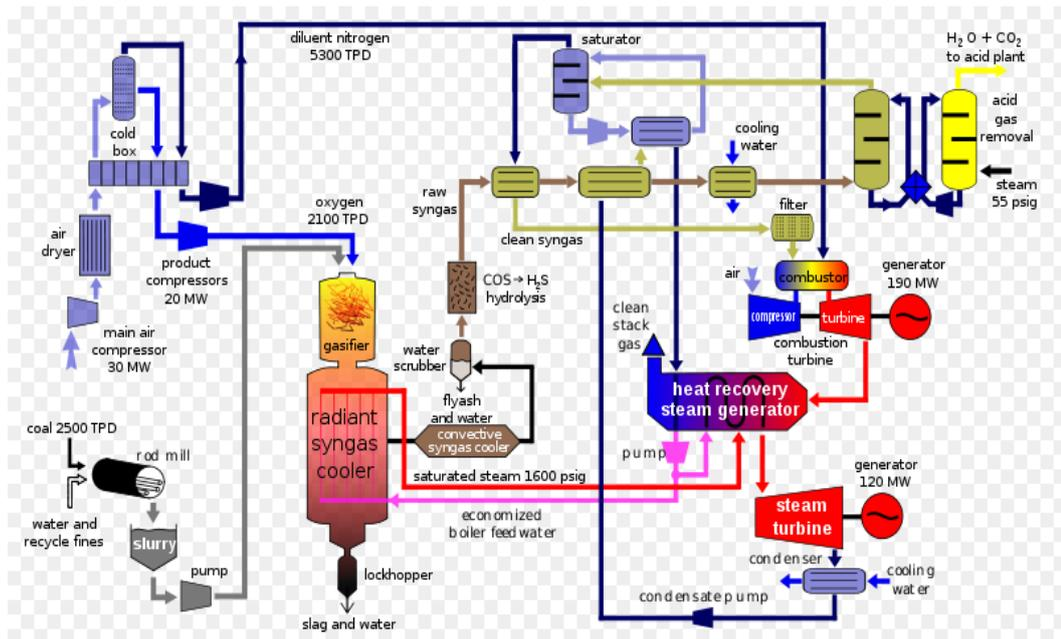
Figure 43 Integrated Gasification Combined Cycle [72]
