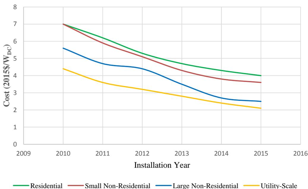
Figure 24 Median Installed Prices of Photovoltaics [14]
