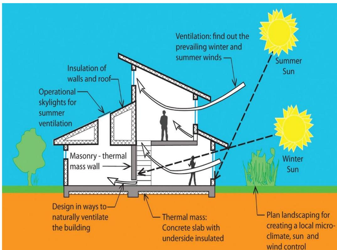
Figure 4 Passive Solar Energy Building Design [22]
