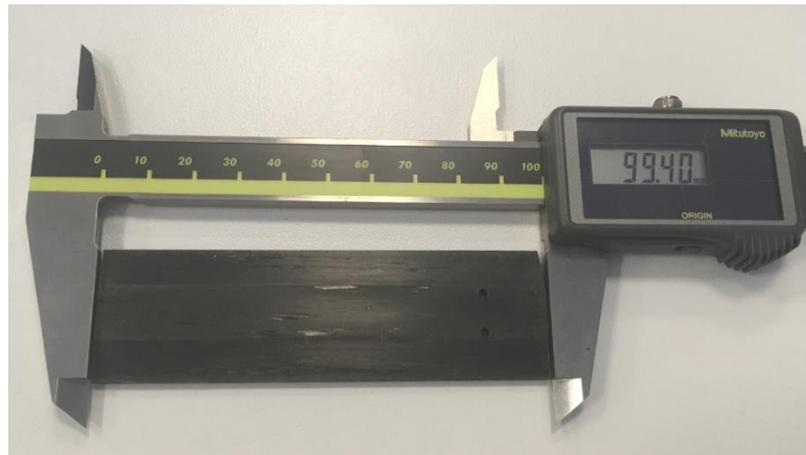
Figure 74 Length of a control surface sample
