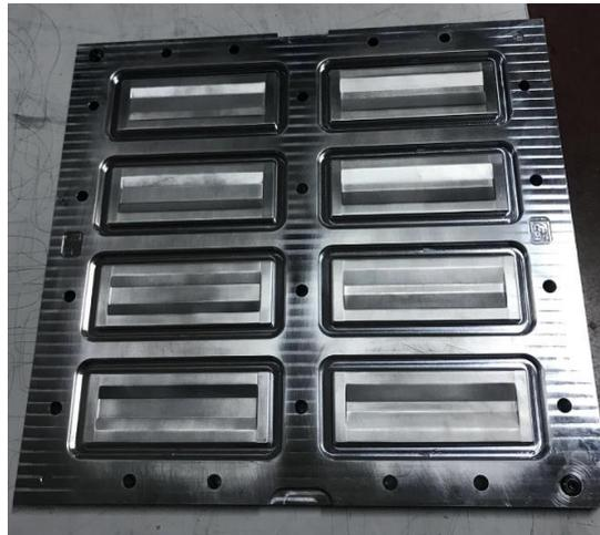
Figure 71 Mould of control surfaces
