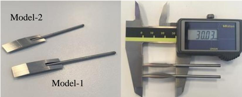
Figure 48 Test specimens and their chord lengths [mm]
