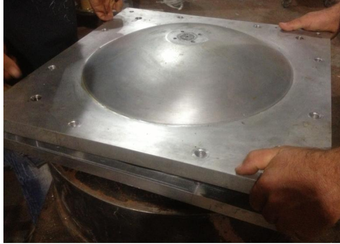
Figure 118: Closing Mold Sections
