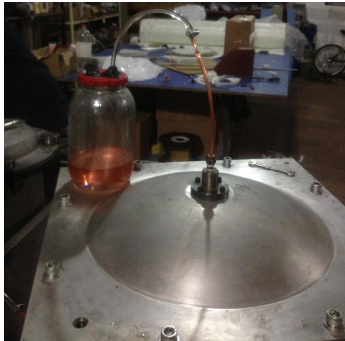
Figure 119: Outlet of Excess Resin
