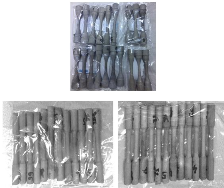
Fig. 3.11 As-cast specimen examples for tensile test
