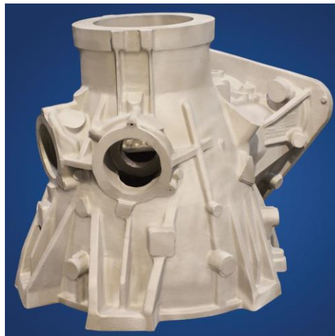
Fig. 1.1 Sikorsky CH53E main casing produced from AZ91 magnesium alloy [22]
