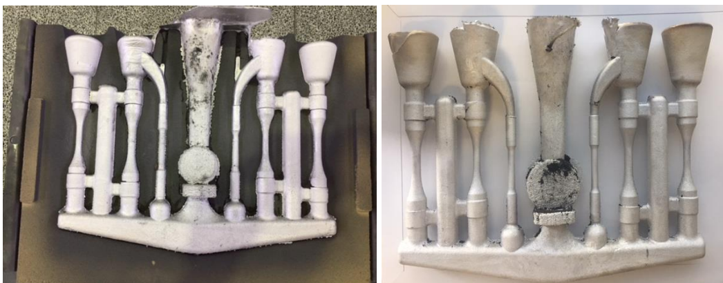
Fig. 3.8 Appearance of the casting bunch after casting in the mould (a) and after moulding cut off
