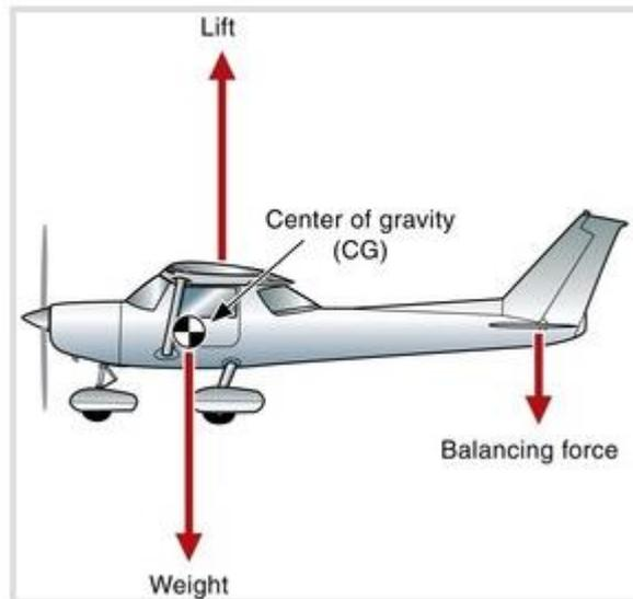
Figure 10 Balancing duty of elevator
