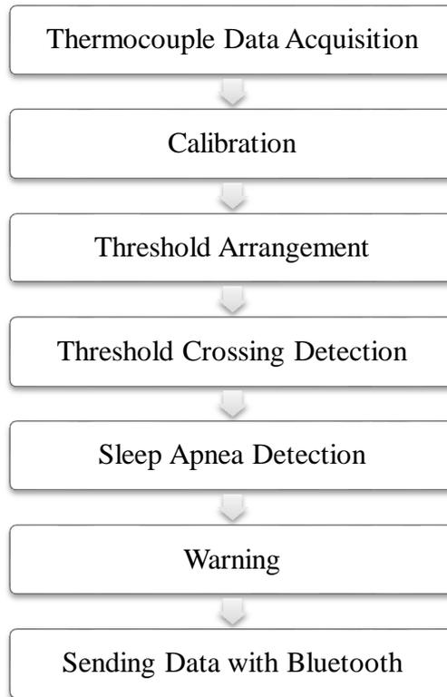
Figure 25 Sleep apnea detection from respiration algorithm block diagram
