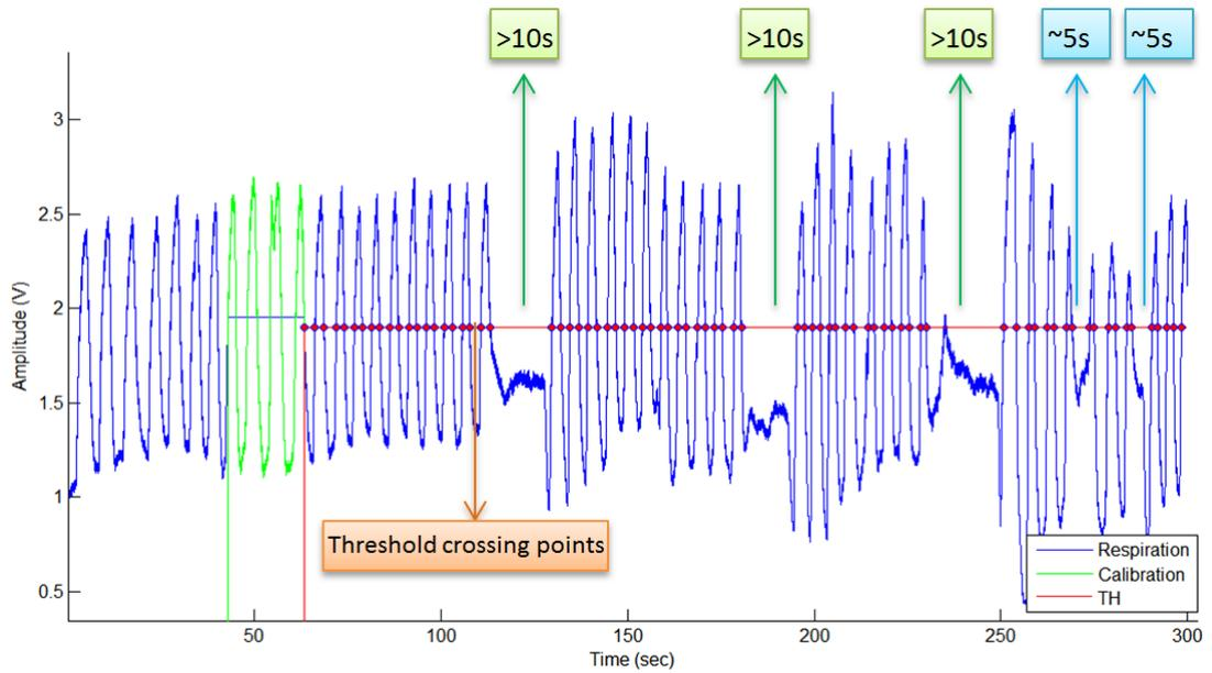
Figure 52 Thermocouple readout recording of Subject-2, blue is thermocouple data, green is thermocouple data during calibration and red one is the threshold value calculated from the calibration signal
