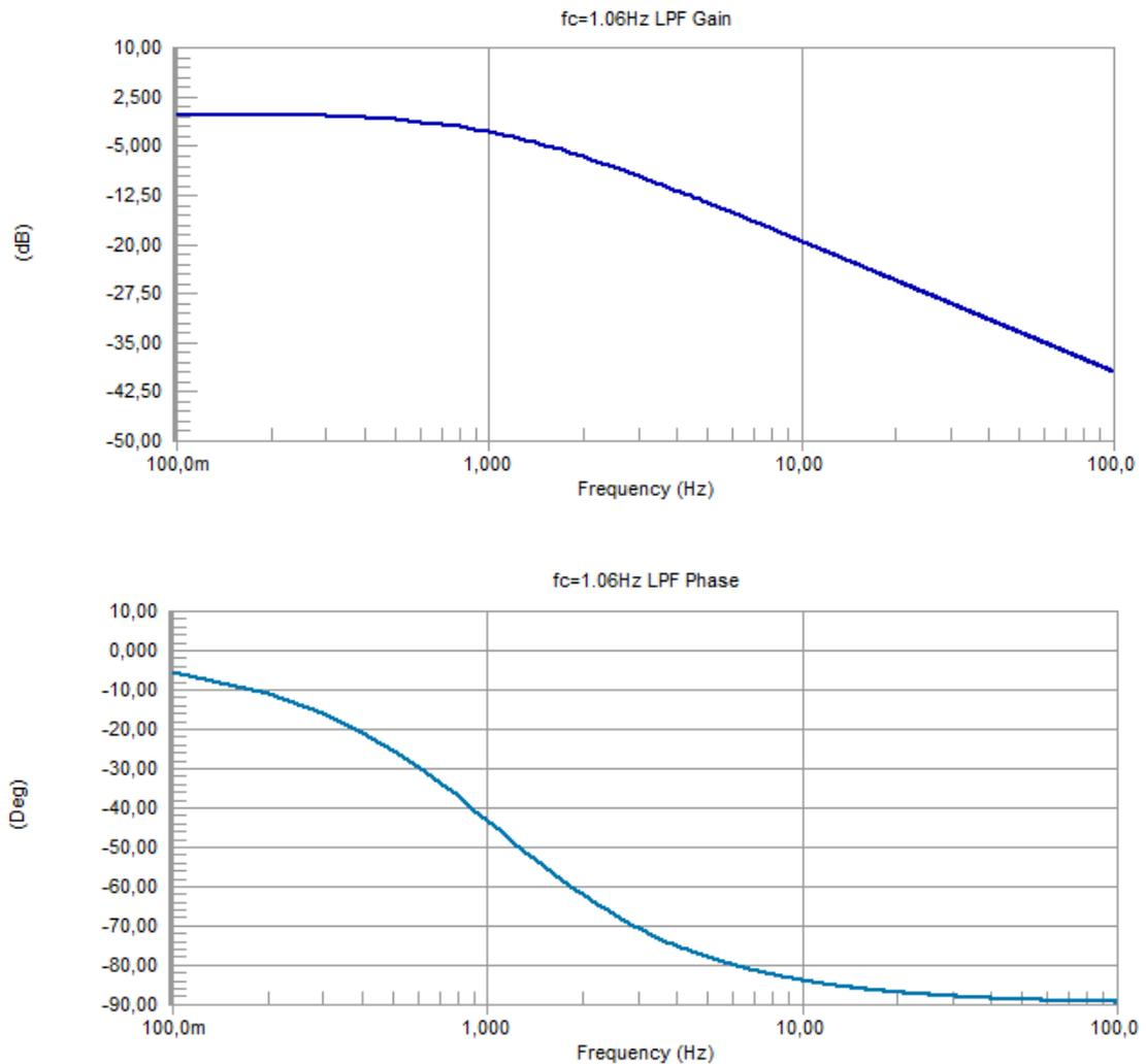
Figure 18 Magnitude and phase response of the low pass filter used in thermocouple analog readout circuit ( $f_c=1.06$  Hz)
