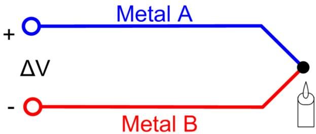
Figure 10 Schematic drawing of a thermocouple
