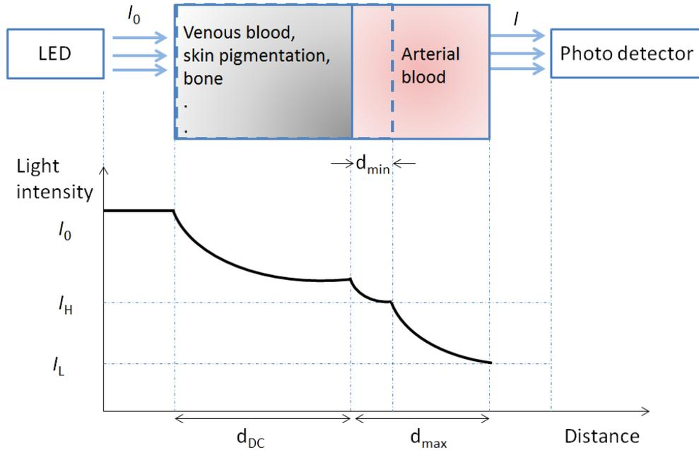
Figure 6 Simplified model of Beer-Lambert's Law in Pulse Oximetry [6]
