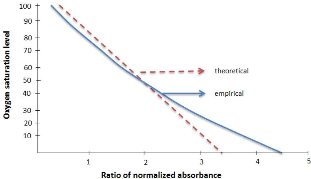
Figure 8 Theoretical versus empirical calibration curves [6]
