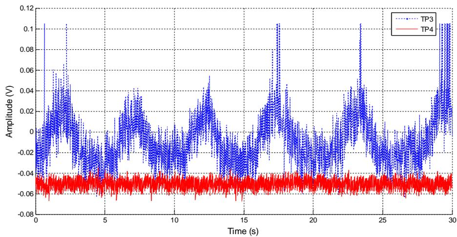
Figure 45 Measurement from TP3 (after high pass filter) and TP4 (after low pass filter) of the pulse oximeter readout circuit
