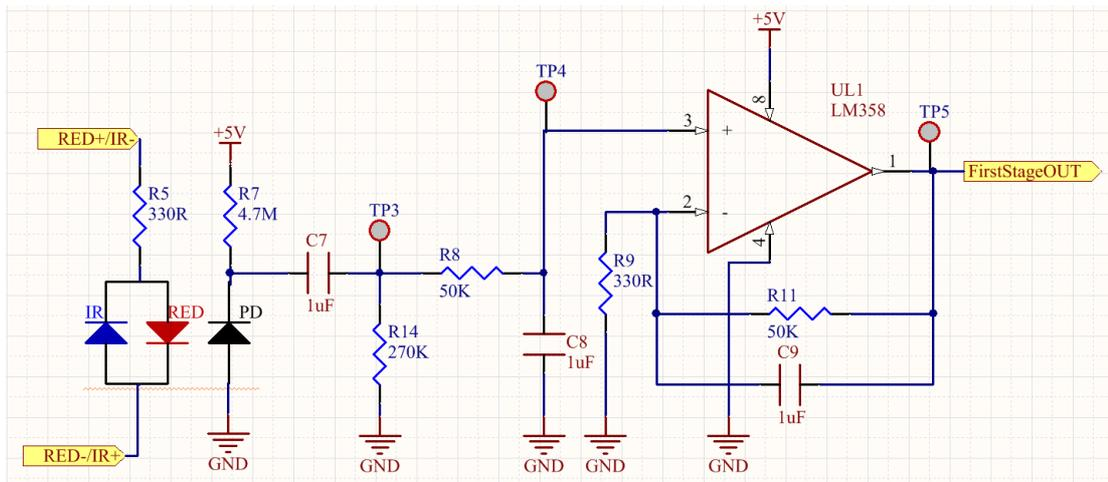
Figure 44 Filtering and first stage amplification circuit of the pulse oximeter readout design
