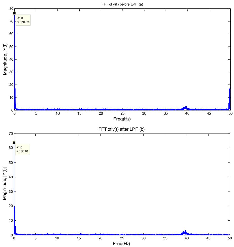
Figure 42 FFT of the respiration signal before LPF (a) and after LPF (b)
