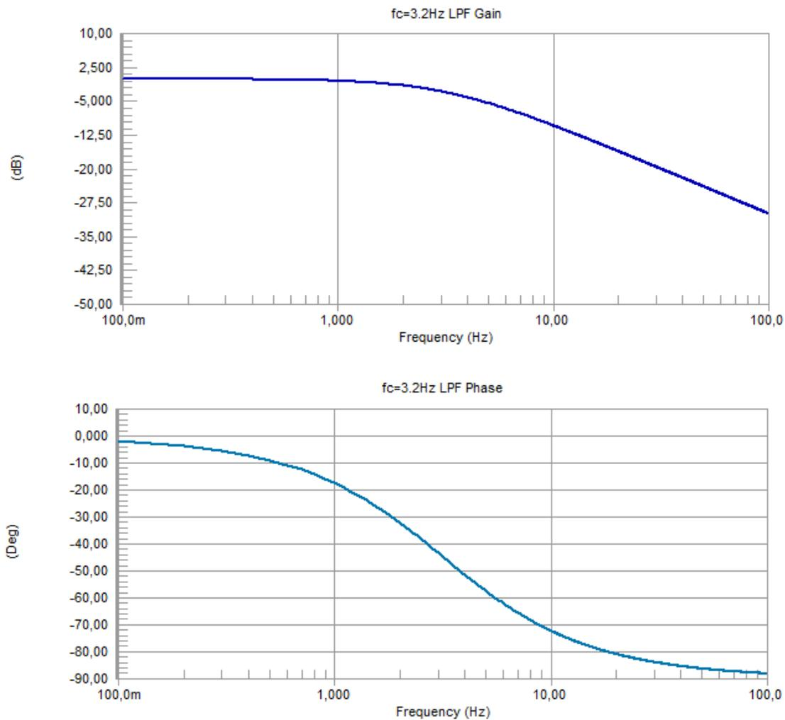
Figure 20 Magnitude and phase response of low pass filter used in pulse oximeter analog readout circuit ( $f_c = 3.2$  Hz)
