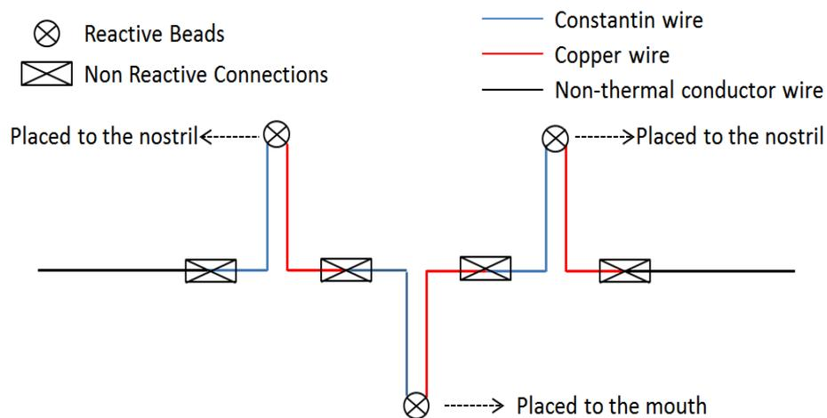
Figure 11 Thermocouple sensor wiring diagram
