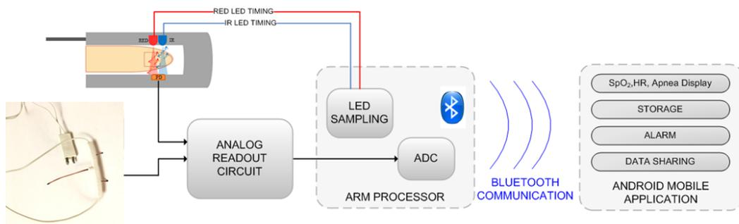
Figure 12 Block diagram of the entire system
