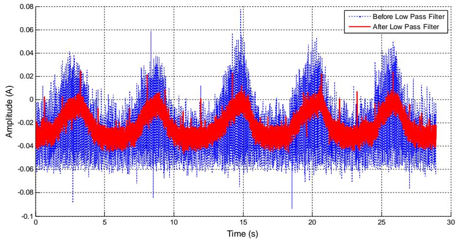
Figure 41 Effect of the low pass filter on the first stage amplification output of the thermocouple readout circuit
