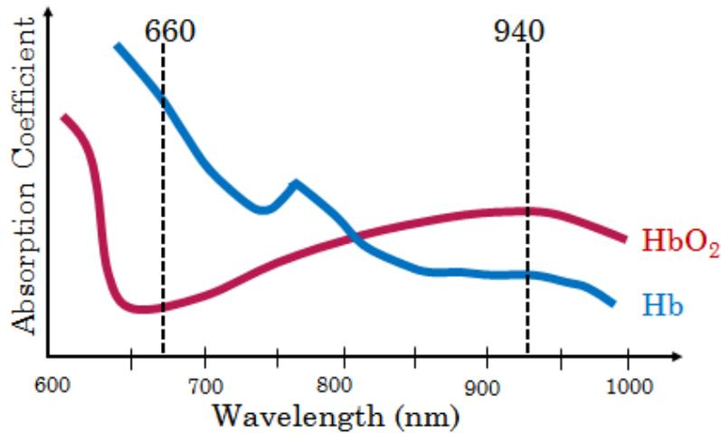
Figure 4 Absorption coefficients of functional hemoglobin species at the wavelengths of interest in pulse oximetry
