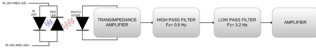
Figure 19 Pulse oximeter readout circuit block diagram
