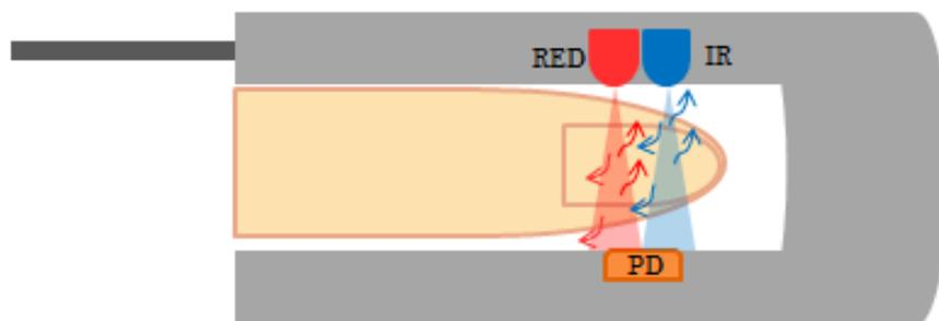
Figure 9 LEDs and photodiode position in the transmission pulse oximeter
