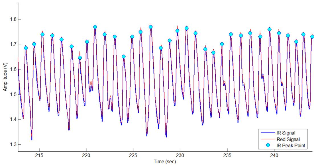
Figure 53 Red and infrared signal obtained from ADC output of the photodiode
