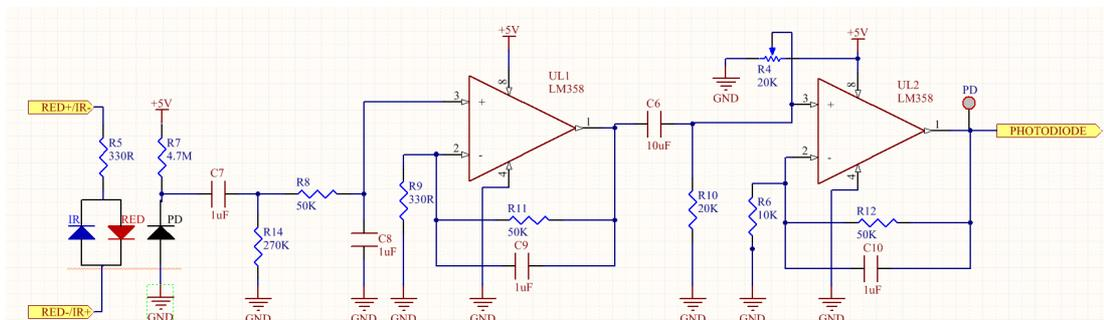
Figure 48 Pulse oximeter readout circuit
