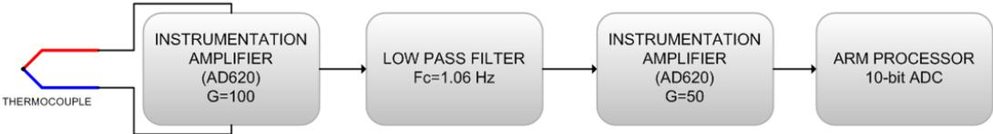
Figure 17 Thermocouple readout circuit block diagram
