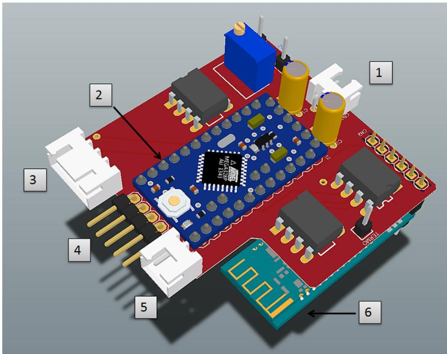
Figure 37 3D visualization of sleep apnea detection system electronic cards and connectors
