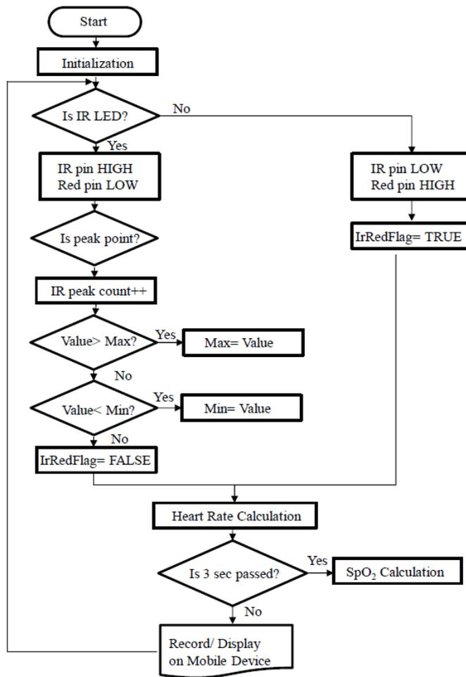
Figure 36 Flowchart of SpO<sub>2</sub> and heart rate measurement
