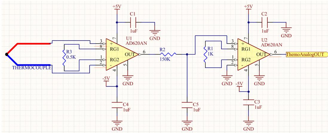
Figure 40 Thermocouple analog readout circuit
