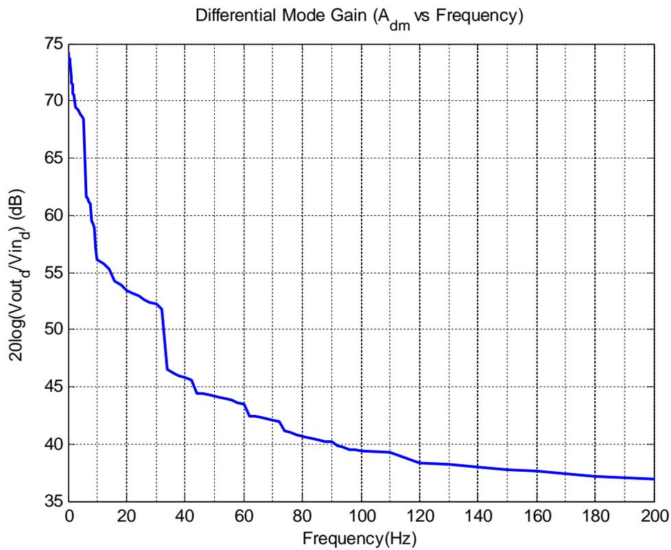
Figure 49 Magnitude response of the thermocouple analog readout circuit
