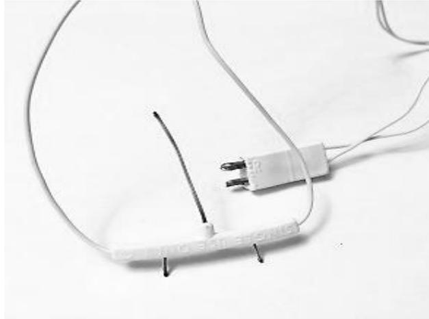
Figure 13 Salter Labs 5800T disposable thermocouple
