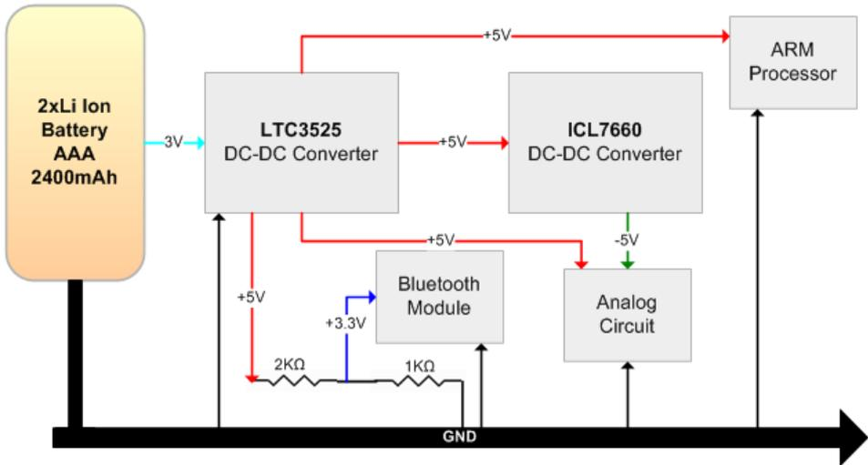
Figure 16 Power circuit block diagram
