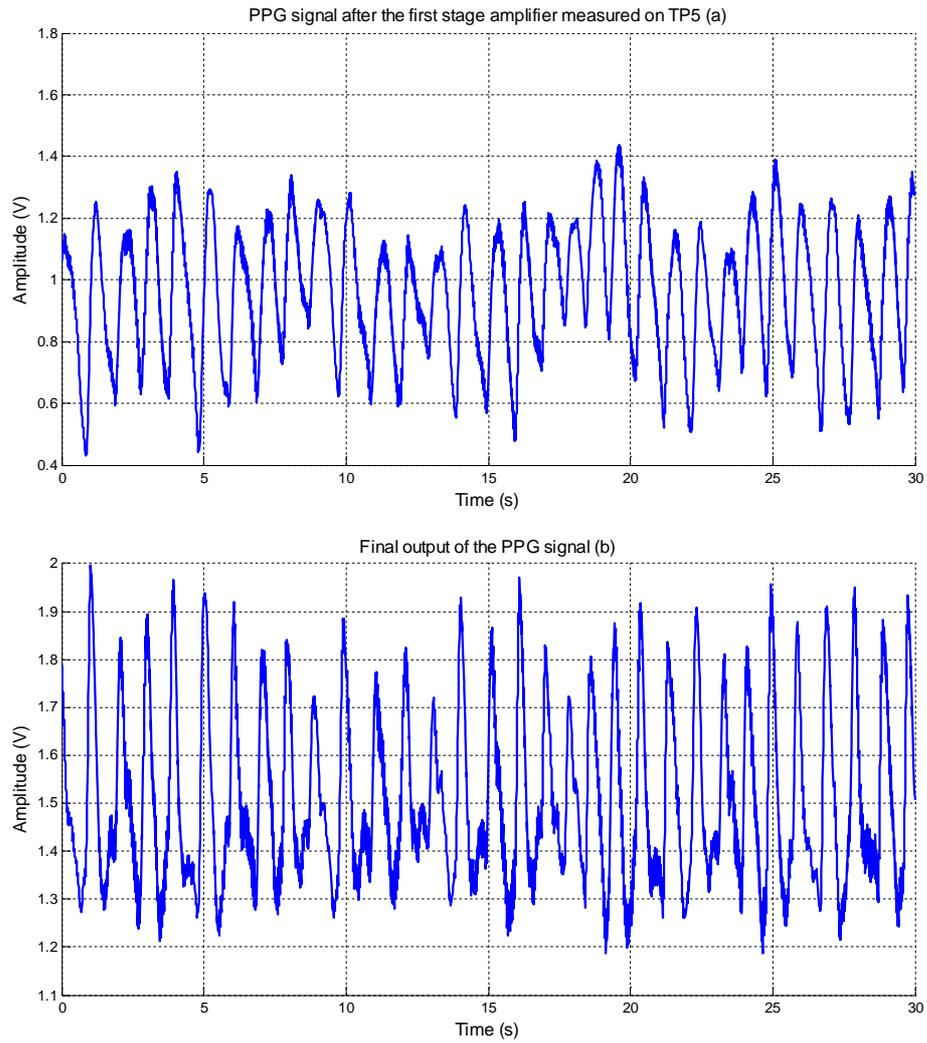
Figure 47 PPG signal after the first stage amplifier measured on TP5 (a), final output of the PPG signal (b)
