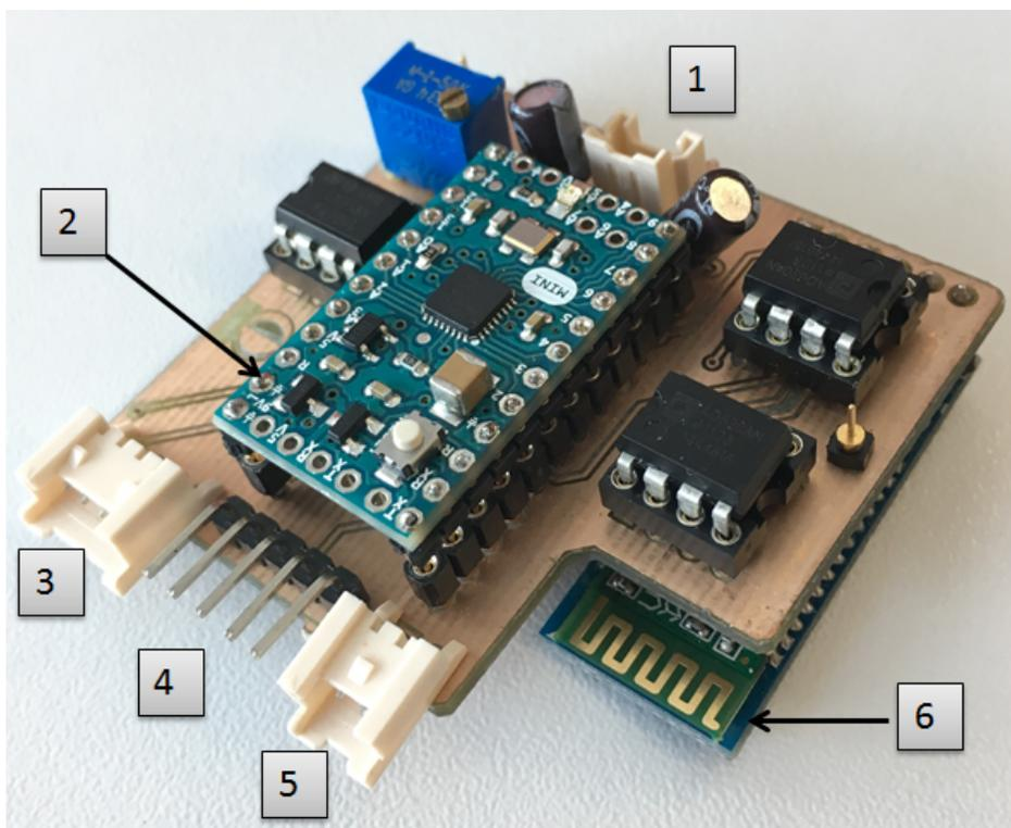
Figure 38 Two layer PCB design of sleep apnea detection system
