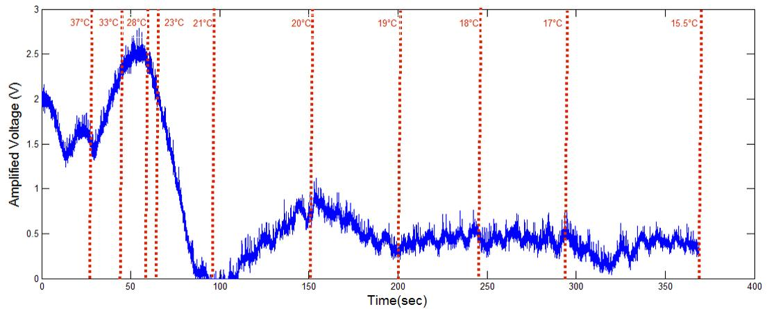
Figure 14 Measured thermocouple temperature response (40°C - 15.5°C)
