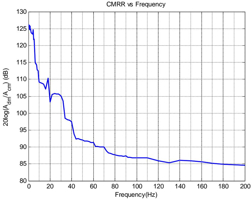
Figure 50 Common Mode Rejection Ratio (CMRR) of the thermocouple readout circuit
