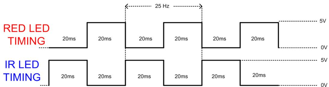
Figure 32 LED timing diagram
