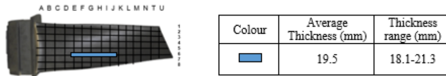
Figure 4.16: The location of samples that were solutionized at 1120°C for 1, 2 and 4 hours and aluminide coated.
