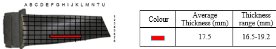
Figure 4.4: The location of samples that were solutionized in between 1080-1235°C for 2 hours and aluminide coated.
