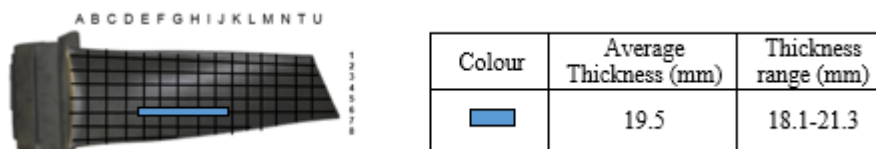
Figure 4.24: The location of samples that were solutionized at 1120°C for 1, 2 and 4 hours and aluminide coated.
