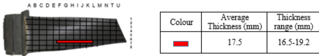
Figure 4.12: The location of samples that were solutionized in between 1080-1235°C for 2 hours and aluminide coated.
