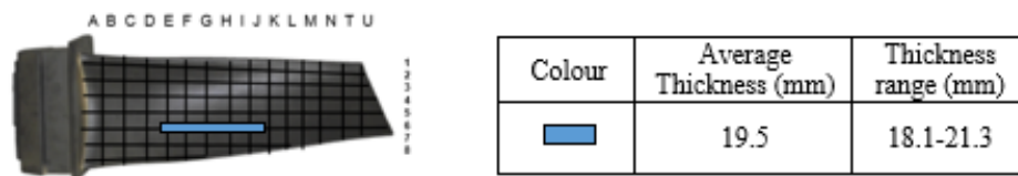
Figure 4.6: The location of samples that were solutionized at 1120°C for 1, 2 and 4 hours and aluminide coated.
