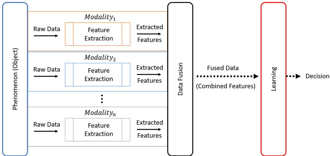
Figure 2.3: A representation of an early fusion structure.
