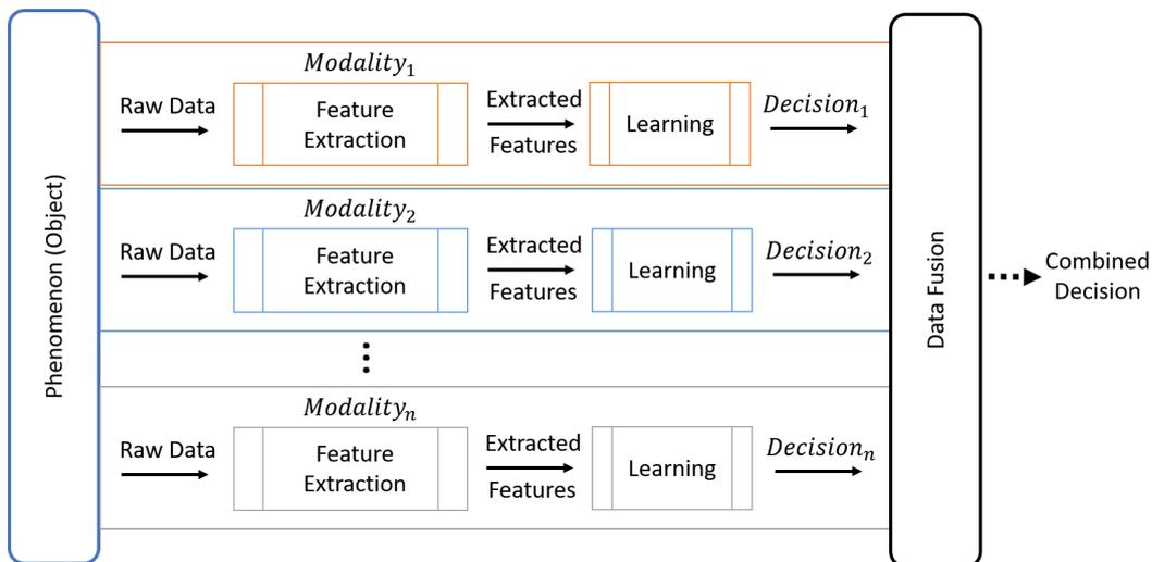
Figure 2.4: A representation of a late fusion scheme.
