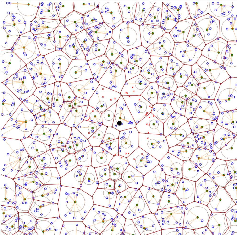
Figure 3.6: A Voronoi graph snapshot of a scene from a WSN clustered by TTDFP.
