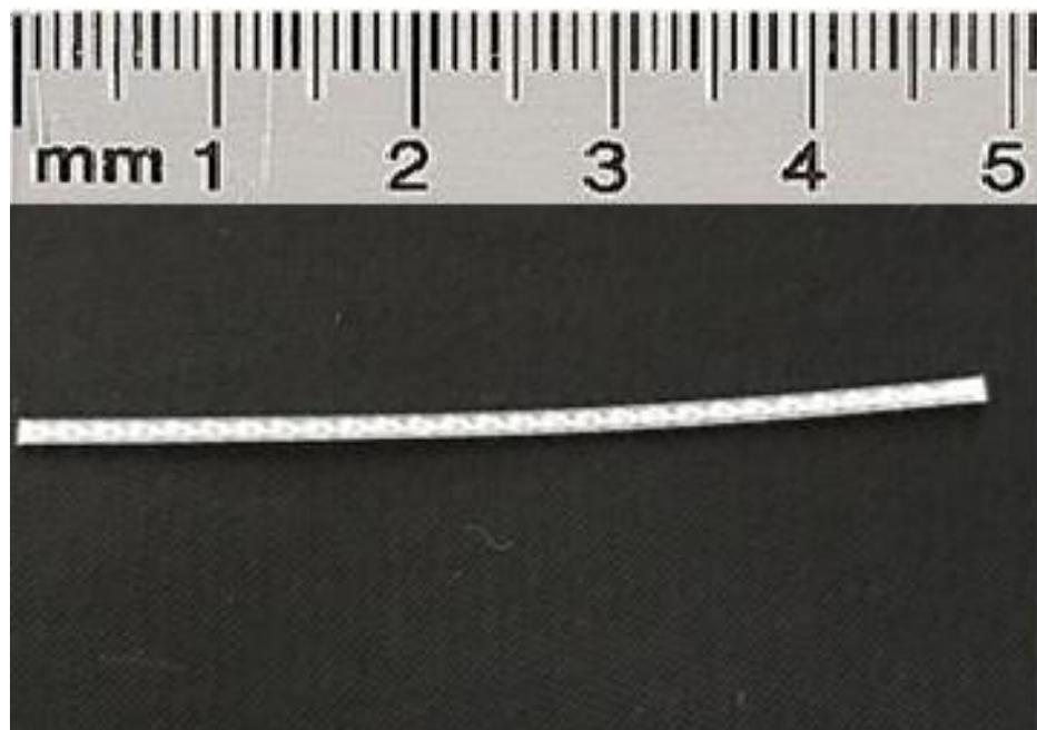
Figure 3.2 Polypropylene fiber used in fiber reinforced mixes
