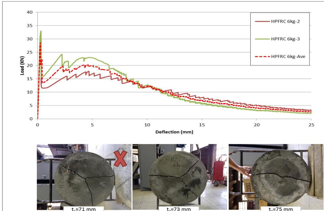
Figure 4.16 Load deflection curves and crack formations of HPFRC 6 kg samples with round panel test for 28 days.
