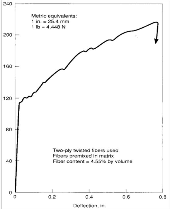
Figure 2.8 Load – deflection graph for concrete containing chopped PP fiber (ACI Committee 544, 2002)
