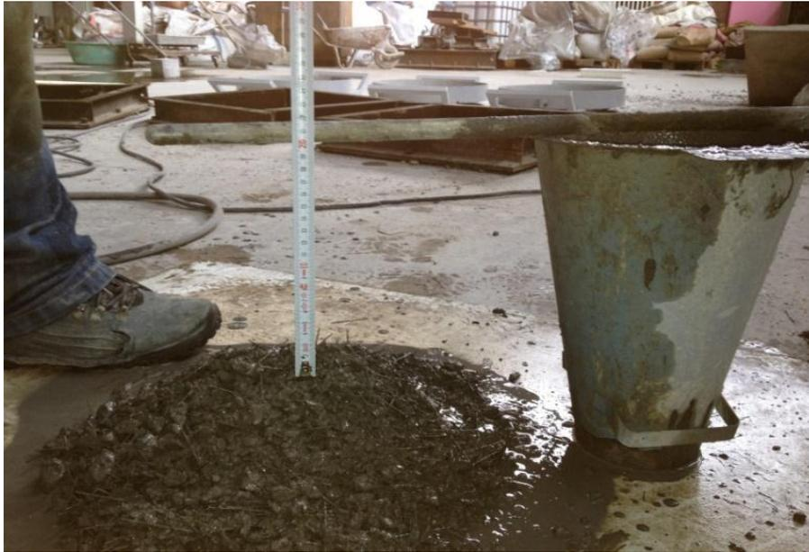
Figure 3.5 Slump test
