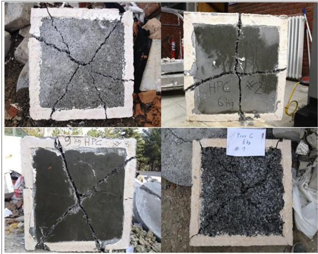
Figure 3.8 Representative pictures of cracked square panels
