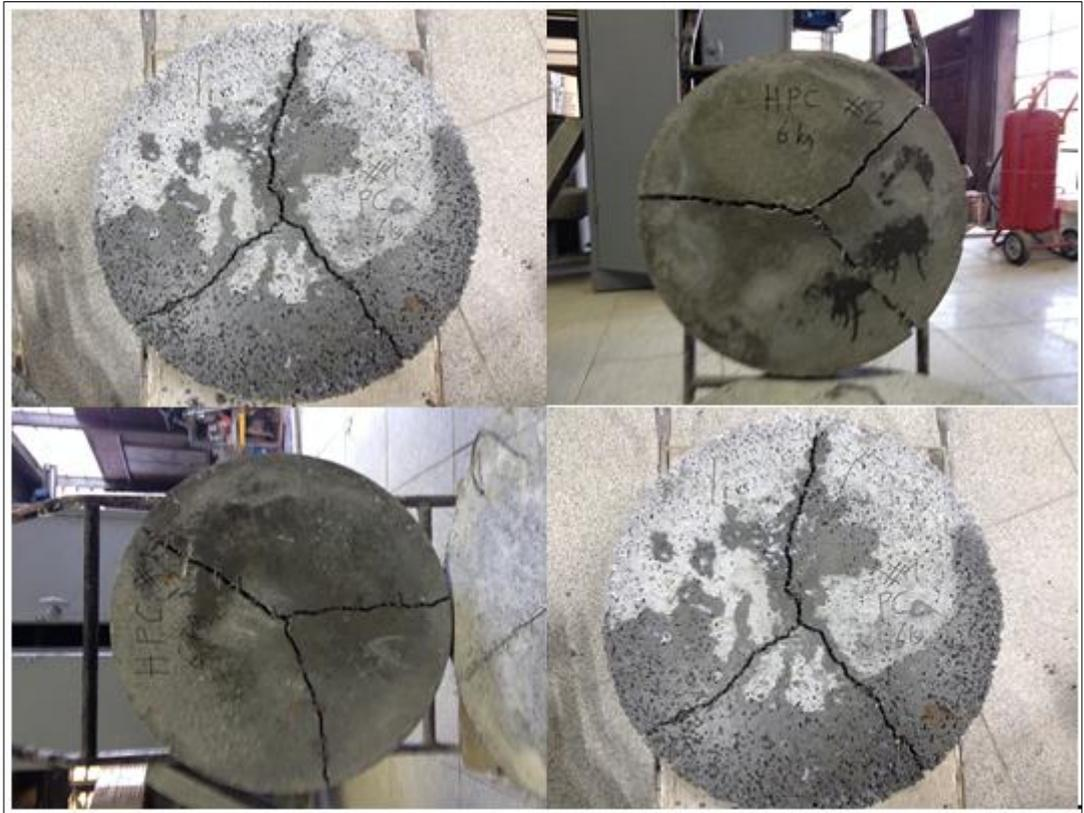
Figure 3.10 Representative pictures of cracked round panels
