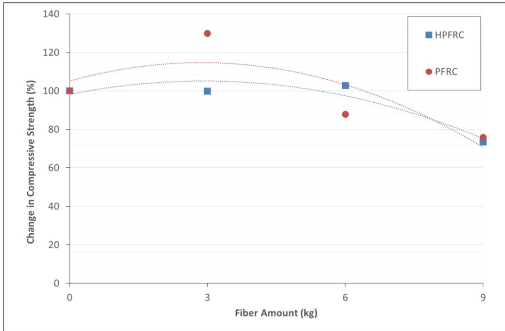
Figure 4.1 Change in compressive strength of all mixes
