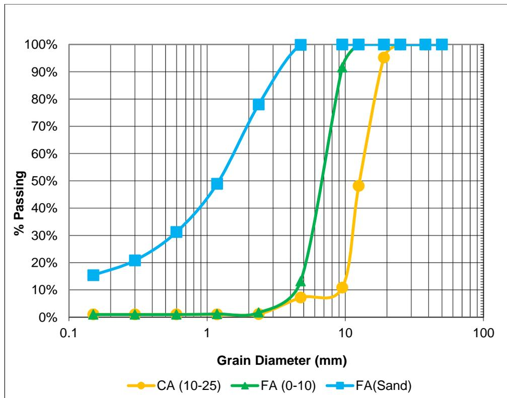
Figure 3.1 Sieve analyses of aggregates
