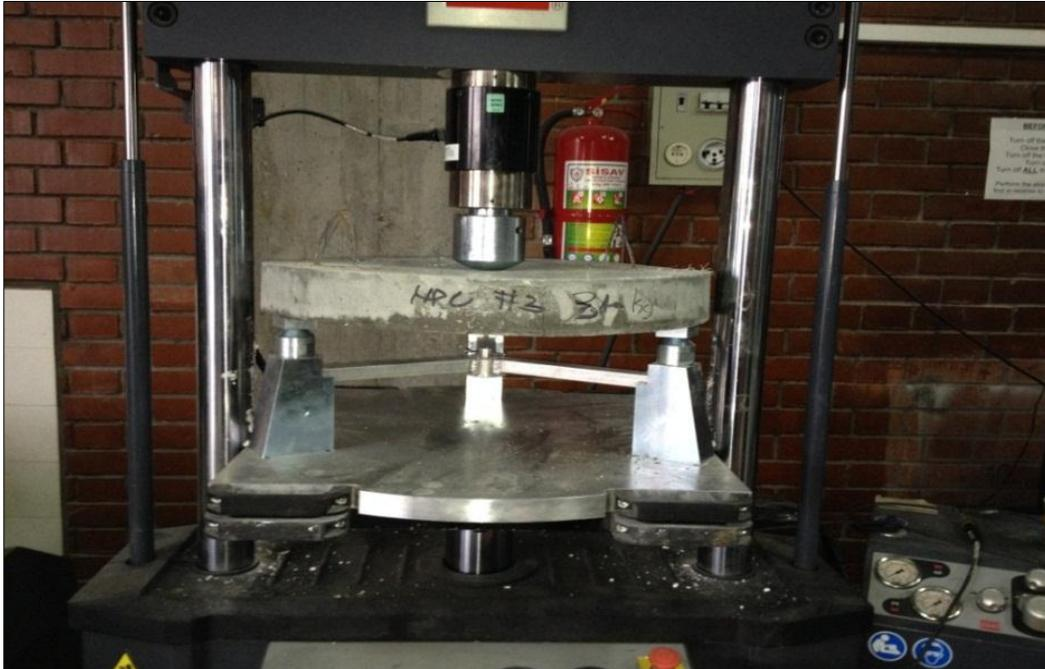
Figure 3.9 Set-up for round panel tests
