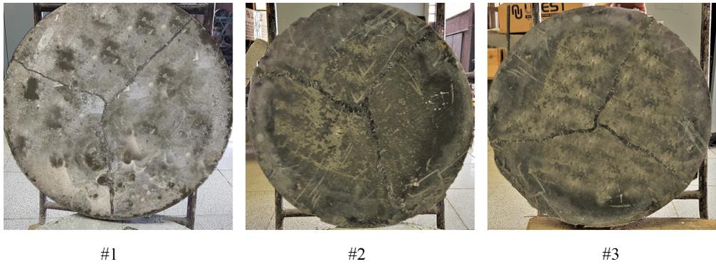
Figure 4.13: Force deflection graph and crack pattern of NPFC 3 round panel samples
