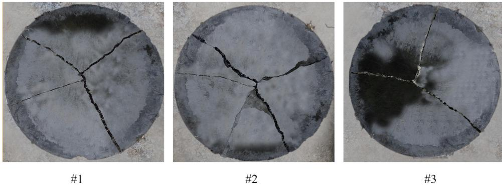
Figure 4.15: Force deflection graph and crack pattern of NPFC 9 round panel samples
