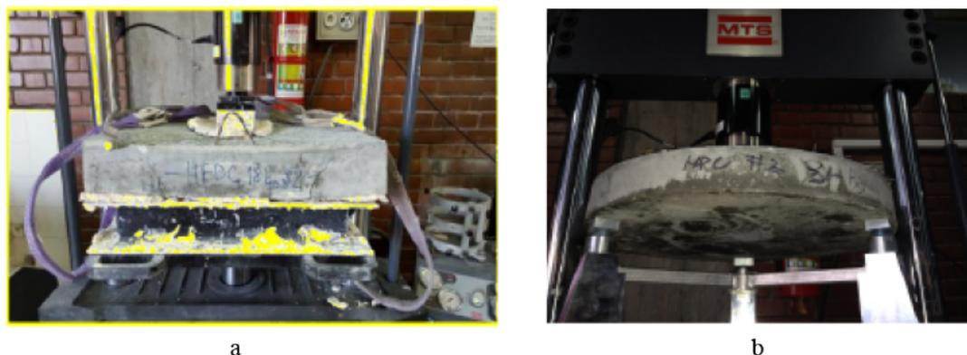
Figure 3.8: The two types of specimen tested a) Square panel b) Round panel
