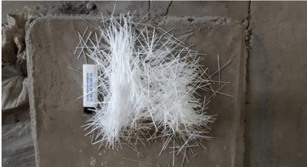
Figure 3.1: Polypropylene fiber used
