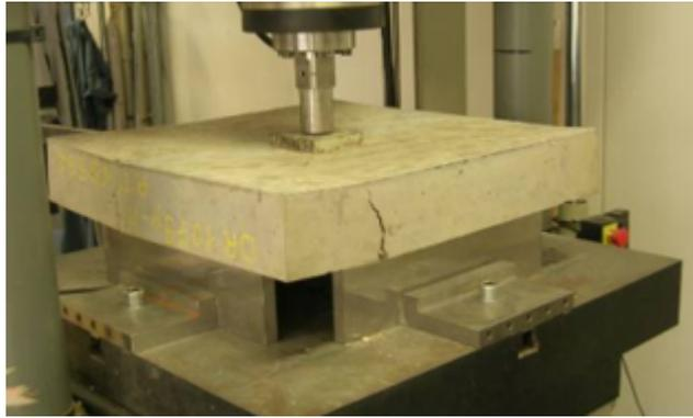
Figure 2.15: ENI14488-5 testing on steel support (Rivaz 2015).
