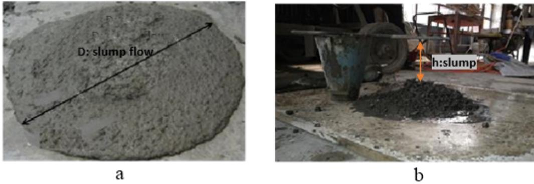
Figure 4.1: a) Slump and b) Slump flow of fresh concrete.
