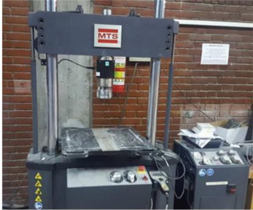
Figure 3.4: MTS testing machine
