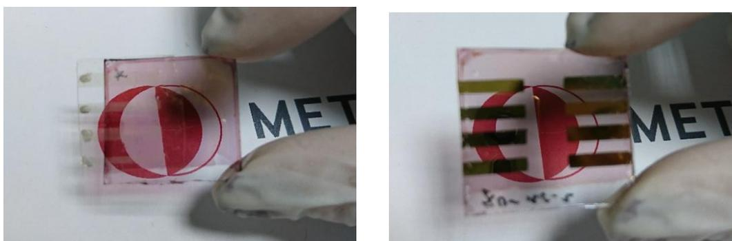
Figure 3. 17 Photographs of an inverted solar cell with Ag NW/PDMS top electrode (left) and Au top electrode (right).
