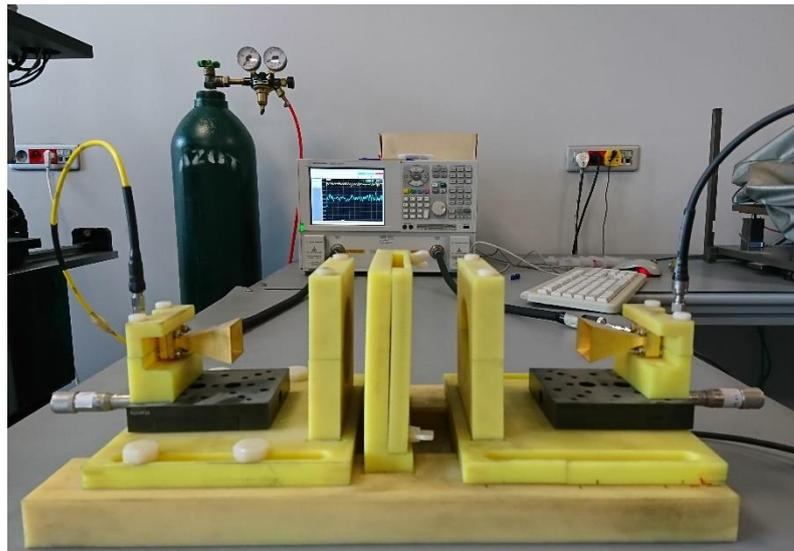
Figure 2. 10 Photograph of free space measurement setup used in this thesis.
