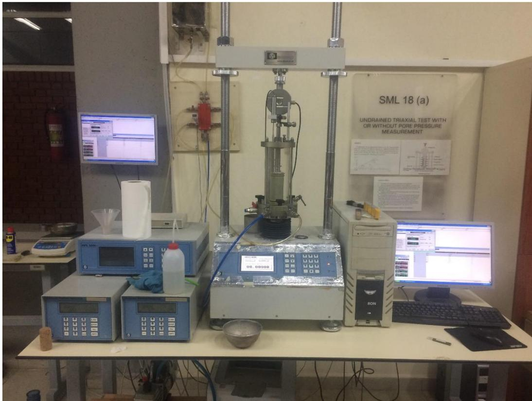
**Figure 3.10. Triaxial testing system used in this study**
