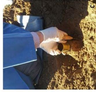
Figure 4-2 Sample point locations (a) and soil sampling procedure (b, c)
