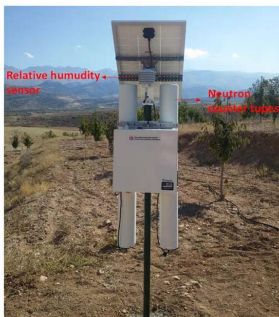
Figure 4-1 Cosmic-ray soil moisture sensor system (CRS 2000/B)
