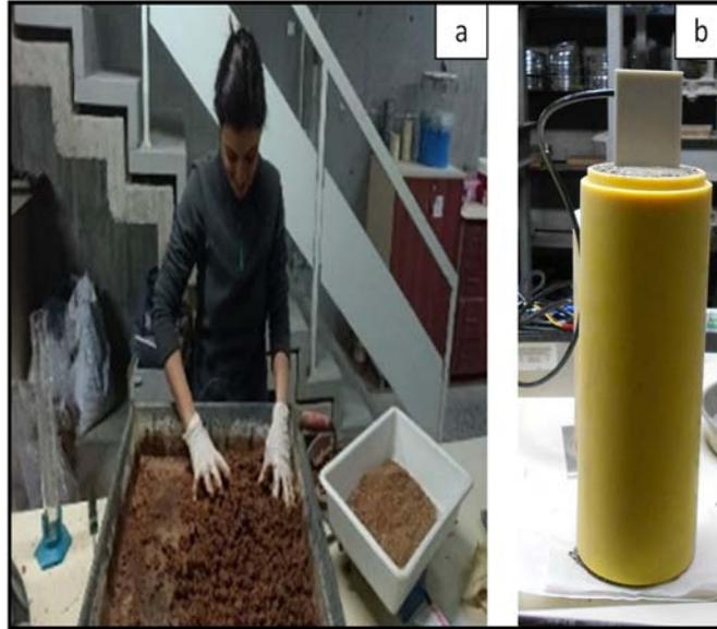
Figure 4-7 Homogeneously wetting (a), CS-616 measurement (b)
