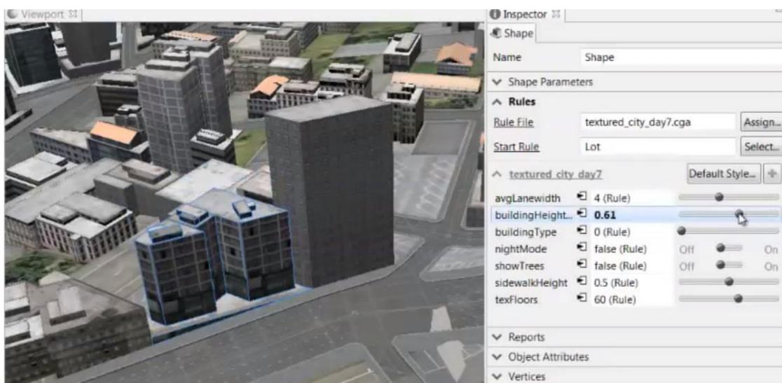
Figure 25: City model produced by ESRI CityEngine and an example control panel for object parameters of selected building. (Retrieved from <http://www.arcgis.com/apps/MapAndAppGallery/index.html> and <http://www.esri.com/software/cityengine/getting-started>; accessed date: 06.06.2017)
