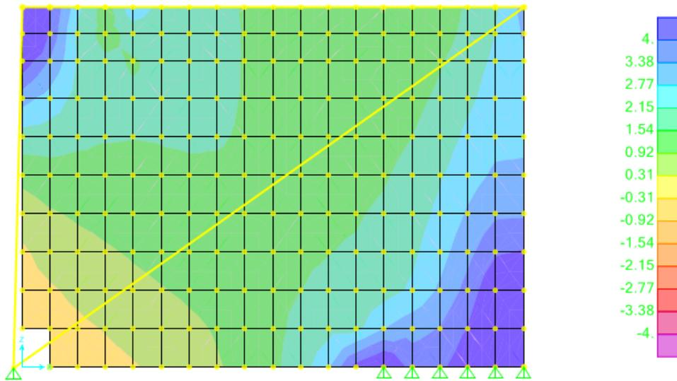
Figure 4.20 SAP2000 stress von-Mises results
