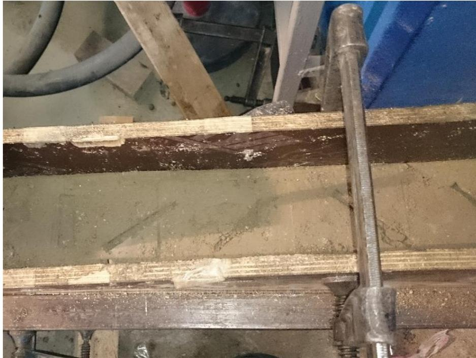
Figure 2.30 Top layer of ramming
