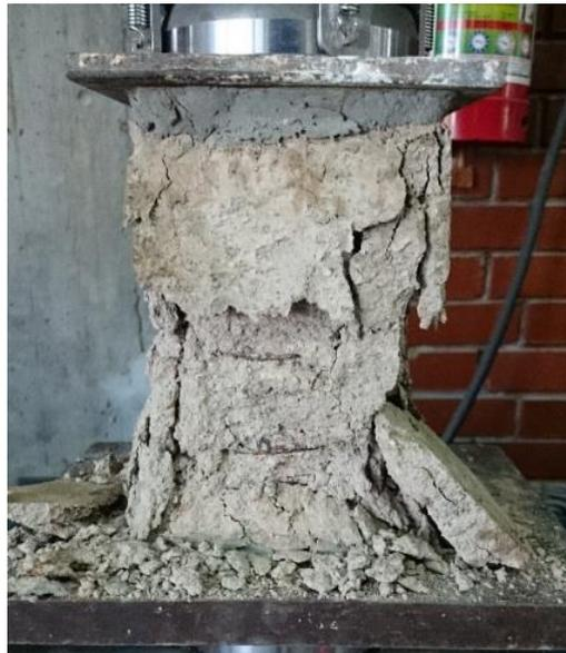
Figure 3.22 Steel hoop confinement column crushing
