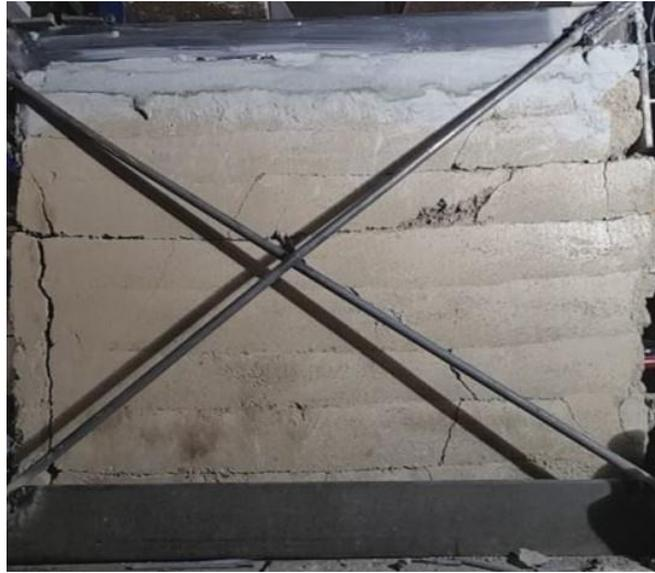
Figure 3.38 Addition of diagonal reinforcements
