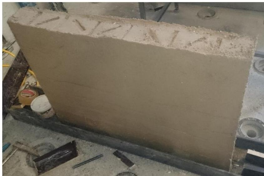
Figure 2.32 REW after formworks were removed
