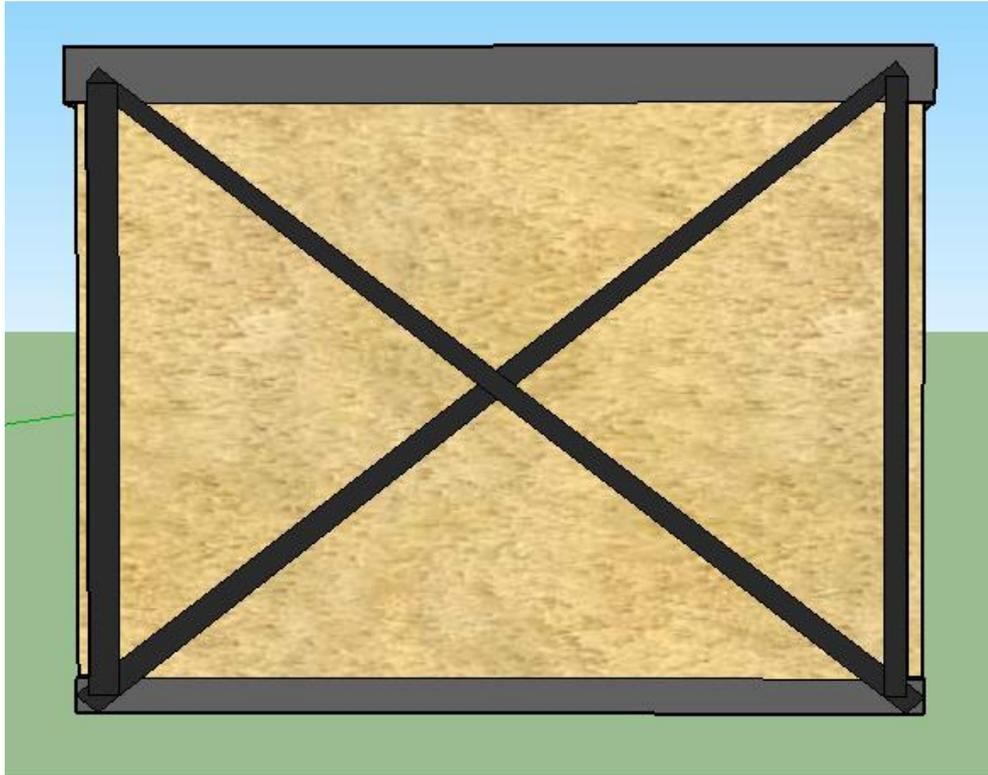
Figure 2.36 REW with vertical + diagonal reinforcement
