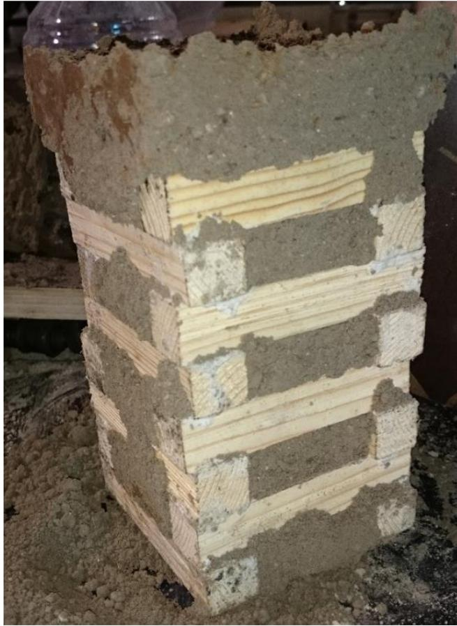
Figure 2.13 Wooden confinement column final view
