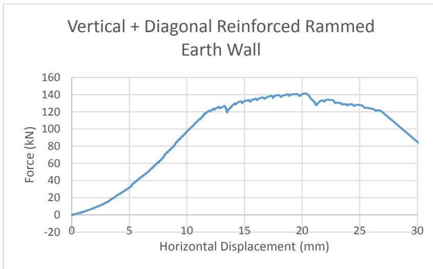
Figure 3.32 Test 1.3 - results of vertical + diagonal RREW
