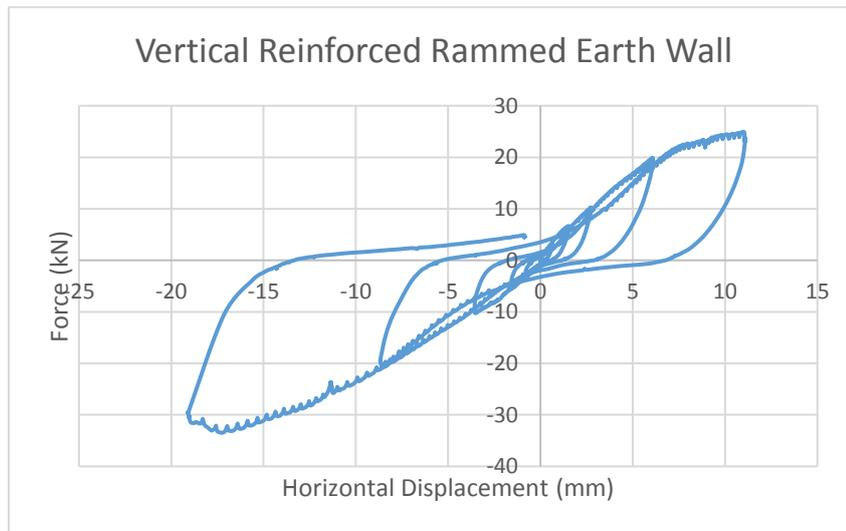
Figure 3.37 Test 2.1 - results of embedded vertical RREW
