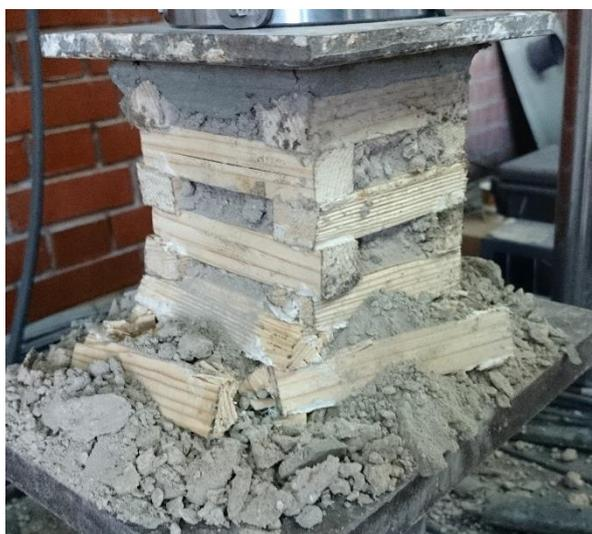
Figure 3.13 Wooden confinement column crushing fail of 2nd level
