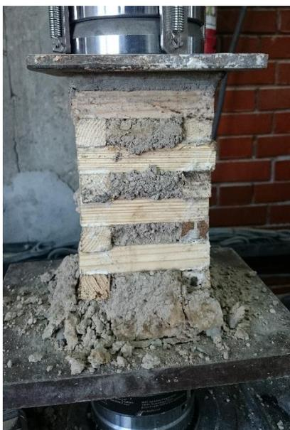
Figure 3.12 Wooden confinement column crushing fail of 1st level
