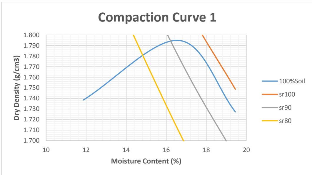
Figure 3.3 Compaction curve of 1st mixture
