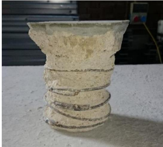
Figure 3.23 Final view of steel hoop confinement column
