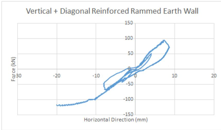
Figure 3.40 Test 2.2 - vertical + diagonal RREW results
