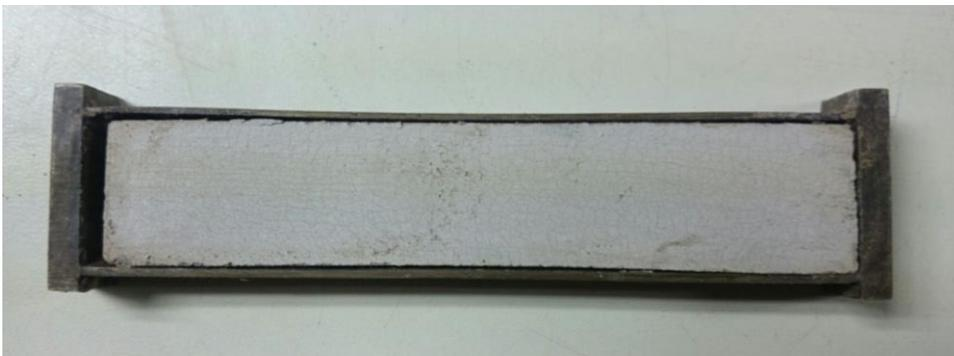
Figure 3.2 Linear shrinkage test sample after drying
