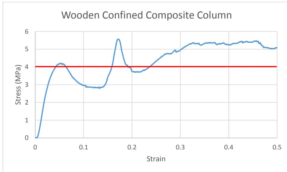
Figure 3.14 Wooden confined column results
