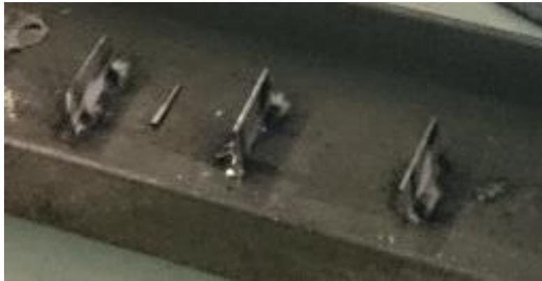
Figure 2.33 Serrations of the bottom profile
