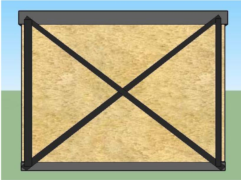
Figure 2.8 REW with vertical + diagonal reinforcement
