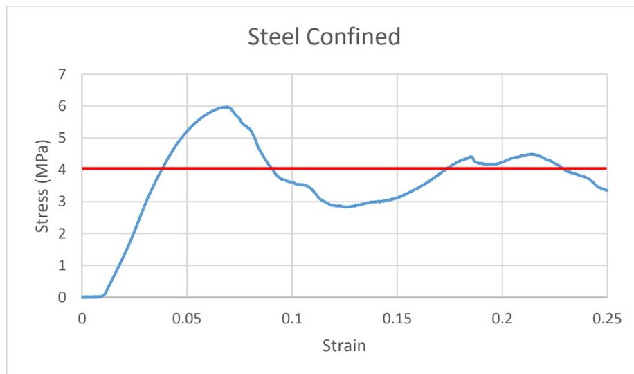
Figure 3.24 Steel hoop confined column test results
