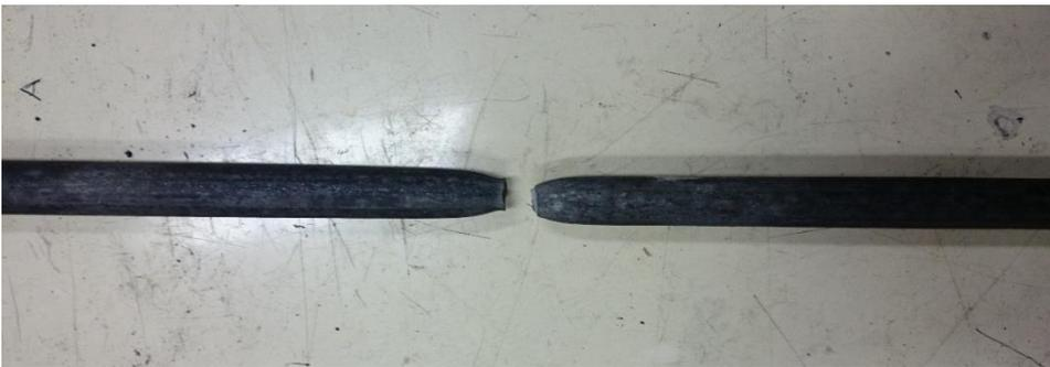
Figure 3.10 Reinforcement bar tensile strength result
