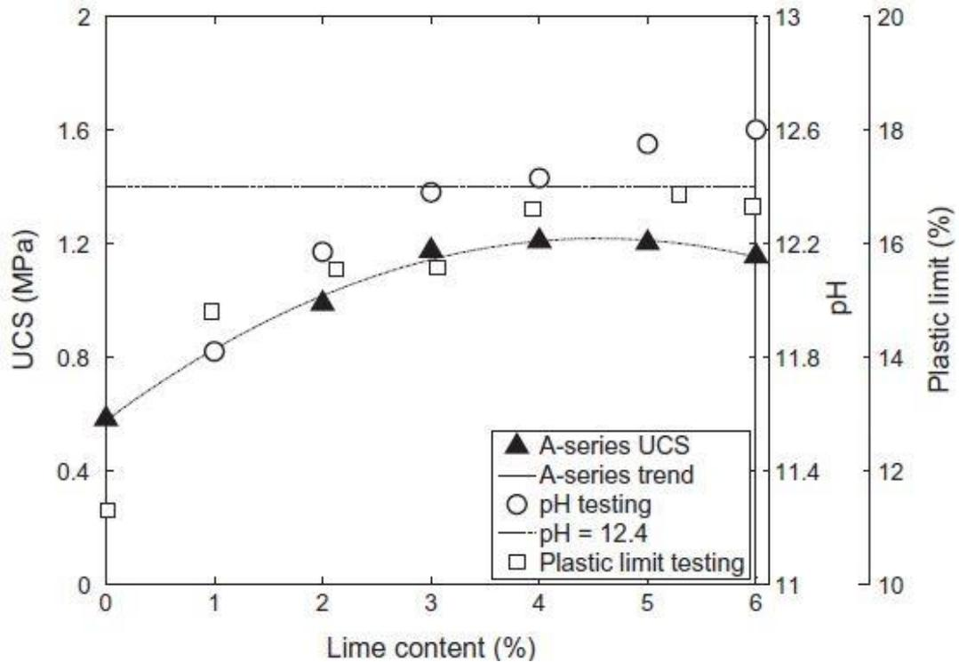
Figure 2.4 Optimum lime content [7]
