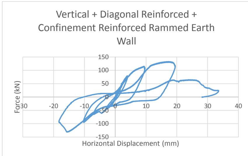
Figure 3.48 Test 3.2 - results of vertical + diagonal RREW with confinement
