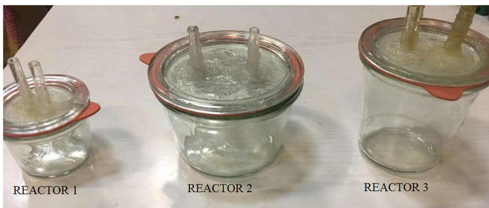
**Figure 12** Reactors used in hydrogen generation from hydrolysis of  $\text{NaBH}_4$
