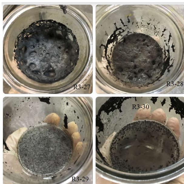
**Figure 34** Picture of the reactor contents after hydrolysis reaction finished
