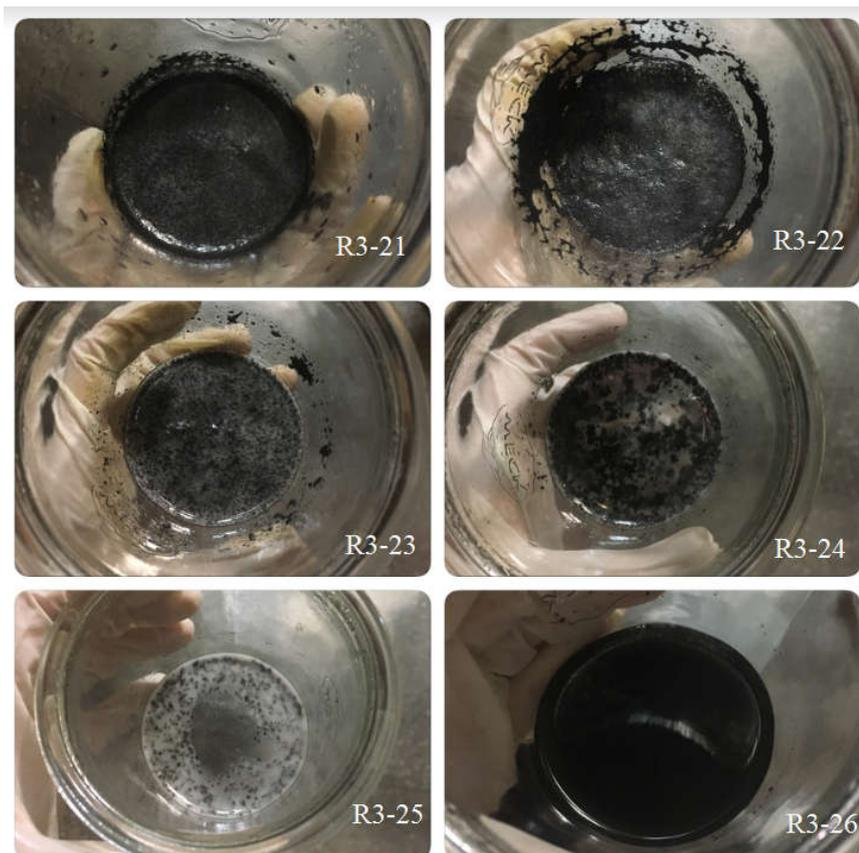
**Figure 31** Pictures of reactor contents for different hydration factors. (5g  $\text{NaBH}_4$  and 0.5g aqueous  $\text{FeCl}_3$  catalyst)
