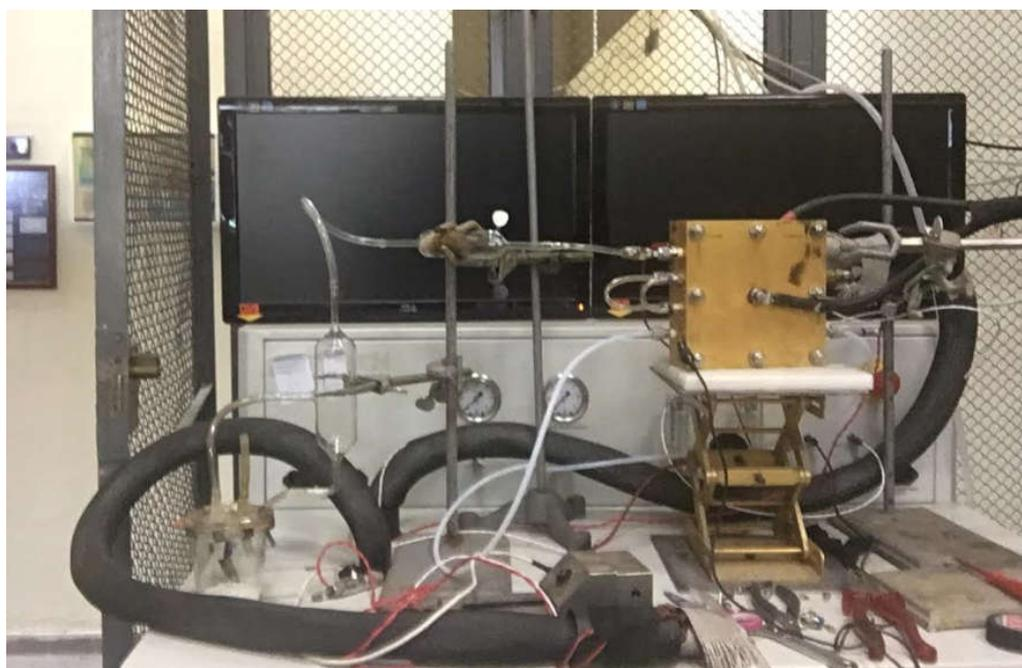
**Figure 54** Integrated  $\text{NaBH}_4$  hydrolysis reactor with one cell PEMFC
