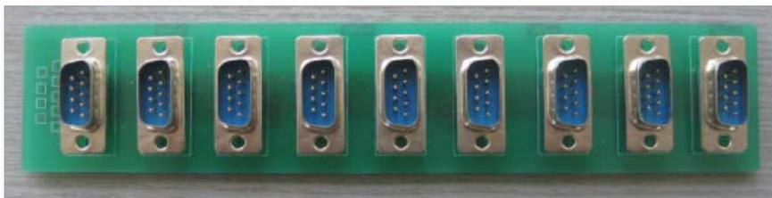
Figure 4.6: The PCB Bus Used for CAN Bus and FlexRay
