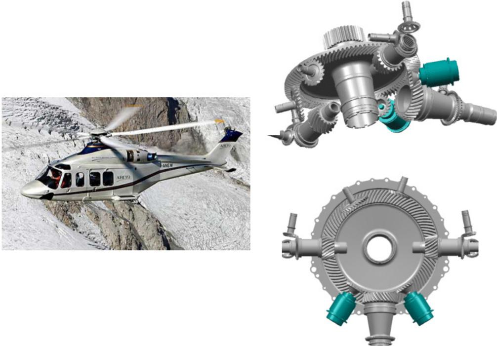
**Fig. 1.4** Collector stage of AW139 helicopter [7]
