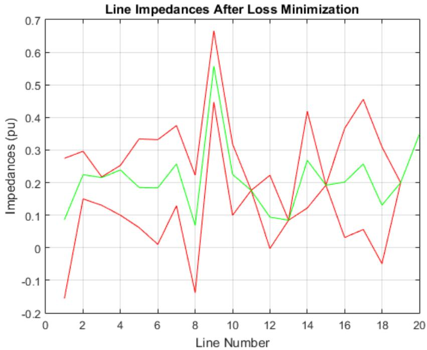
*Figure 33 IEEE 14 Bus System under 50% Load Line Impedances and Impedance Limits after Loss Minimization*
