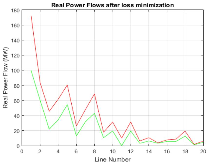
Figure 25 IEEE 14 Bus System under 70% Load Real Power Flows After Loss Minimization
