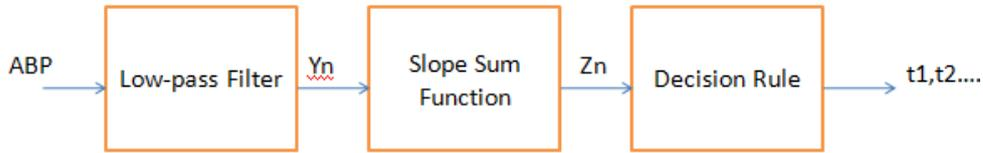
Figure 2.15: Block Diagram of The ABP Onset Time Detection Algorithm
