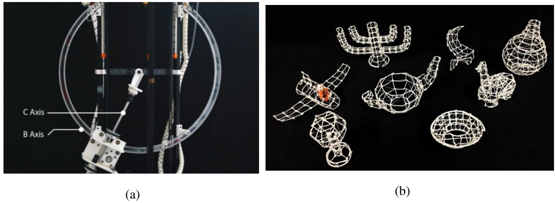
Figure 4.10: 5 DOF WireFrame Printer and its products [2]
