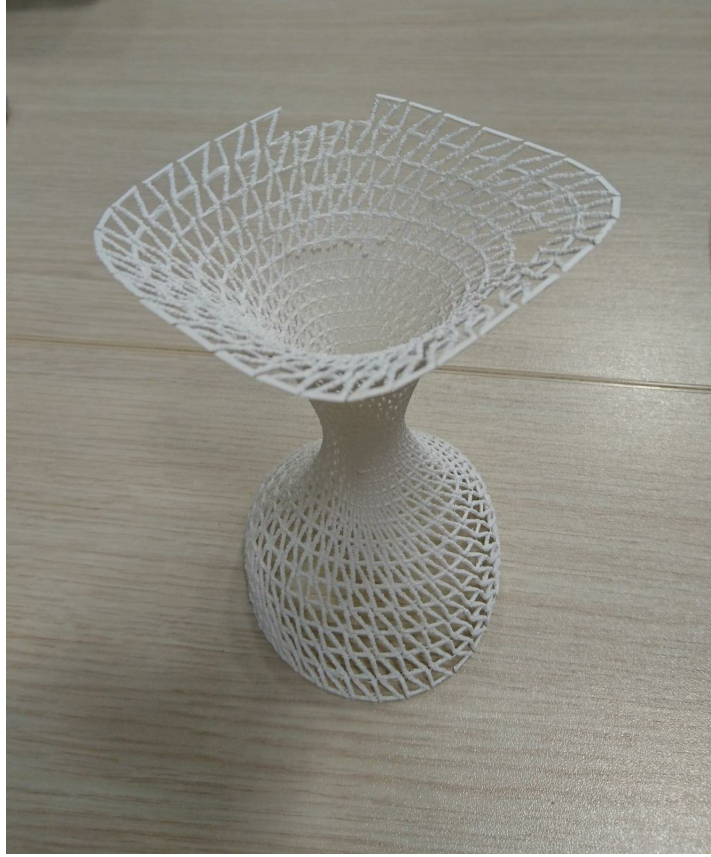
Figure 4.5: Successfully 3D printed auxetic patterns with Ultimaker 2+
