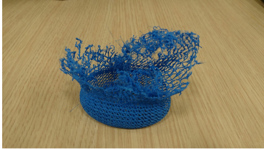
Figure 4.4: Downfall happened while 3D printing with Ultimaker 2+
