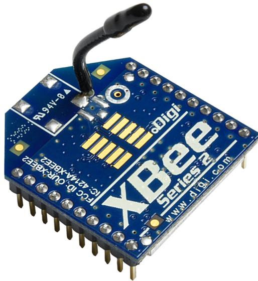
Figure 2.3: XBee Hardware Device [17]
