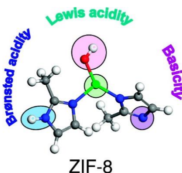
Figure 2. 18 Possible functionality of external surface structure of ZIF-8. Color of atoms are presented in; Zn (green), C (grey), N (blue), H (white), O (red) (Chizallet & Bats, 2010)
