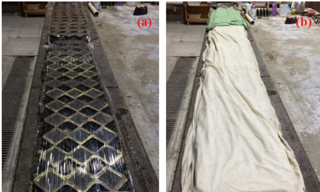
Figure 3.3 Curing of 50-mm cube specimens (a) covered with plastic wrap, (b) covered with a wet cloth
