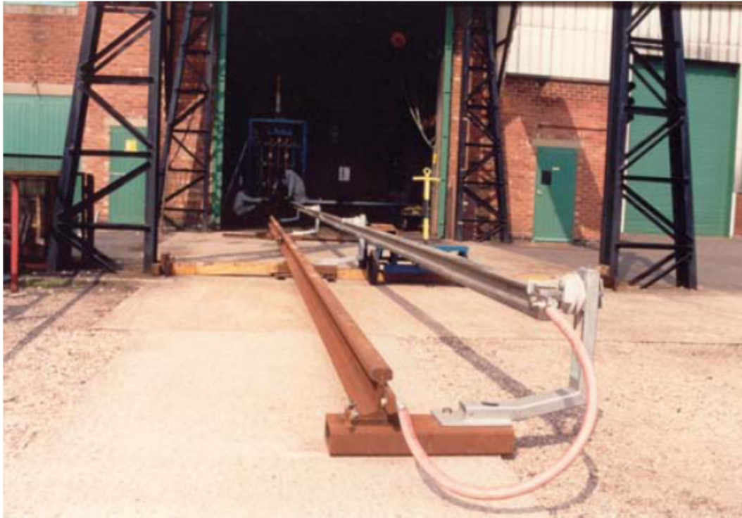
Figure 2.12: An Example of Short Circuit Test of Catenary Line and Return Rail
