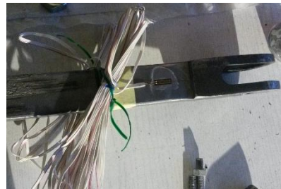
Figure 4-12. Strain gauges installed on a driven bar
