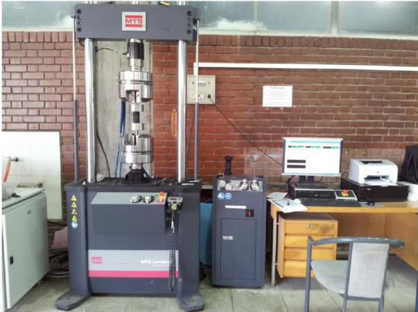
Figure 4-2. MTS Servohydraulic test machine
