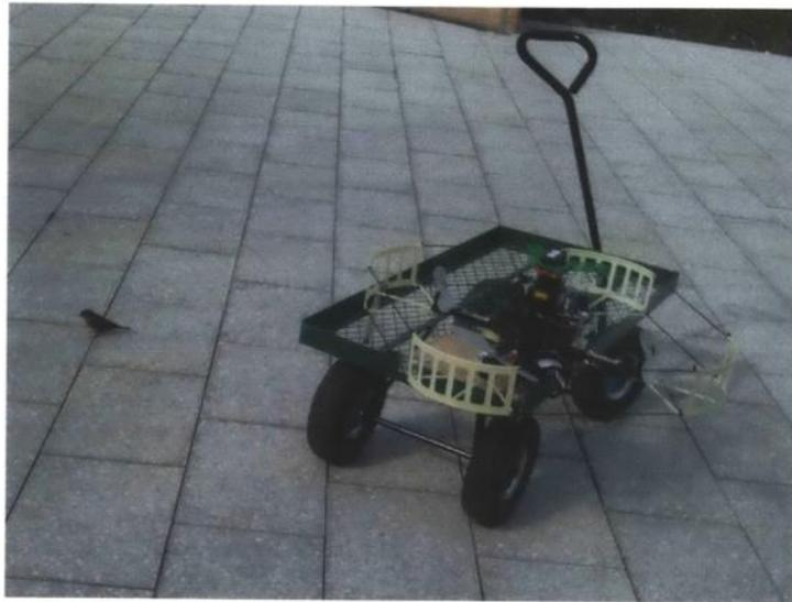
**Figure 2.7** Image of the quadrotor mounted on a cart for data collection
