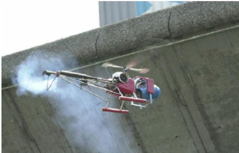
**Figure 2.6** Mono camera integrated helicopter developed for bridge inspection
