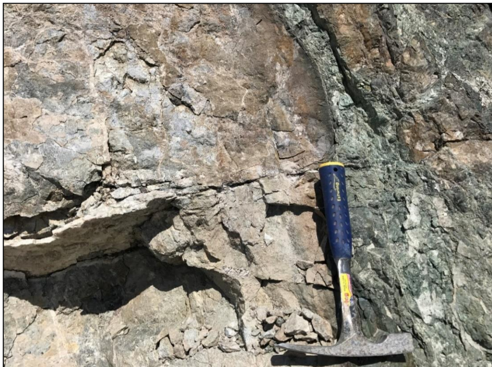
Figure 13. Field photograph of an ultramafic host rock cross-cut by a diabase dyke having chilled margin.
