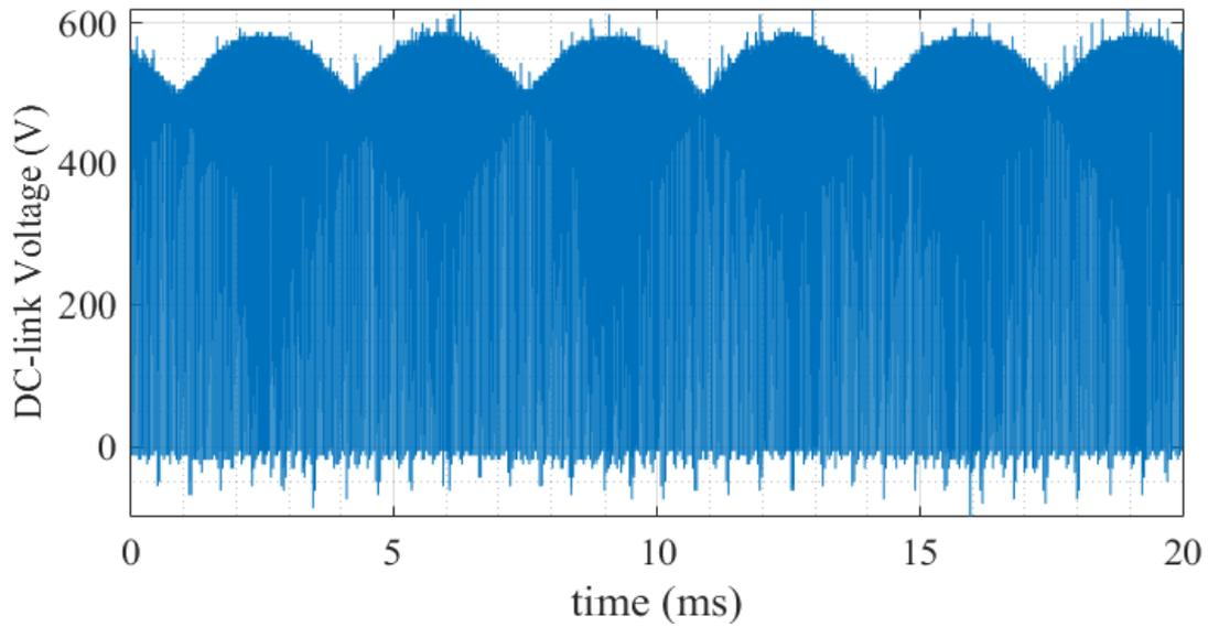
Figure 4.9 DC-link voltage waveform at  $m=0.83$ , sampling rate 25MS/s
