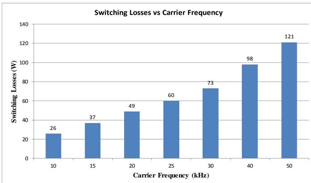
Figure 3.7 Switching losses for different carrier frequencies
