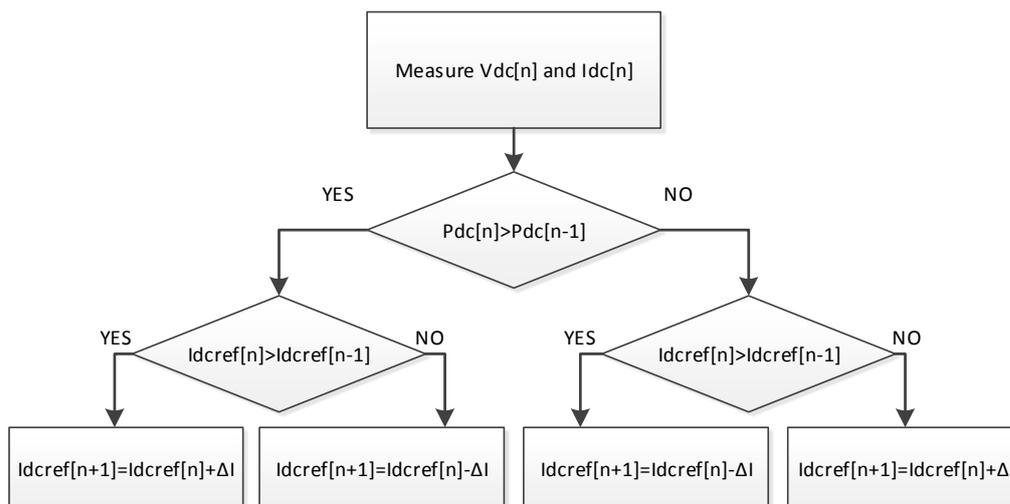
Figure 2.9 Flowchart of the Perturb and Observe algorithm
