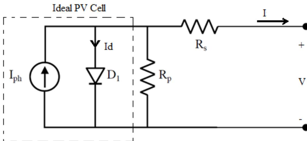
Figure 2.4 Equivalent circuit of a practical PV device
