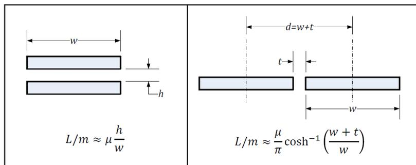
Figure 3.34 Stray inductance approximation for stacked and coplanar PCB traces [79]
