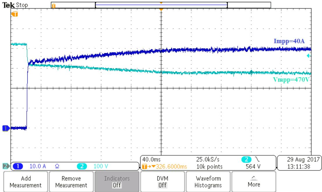
Figure 4.11  $I_{pv}$  (blue) and  $V_{pv}$  (light blue) waveforms during start-up
