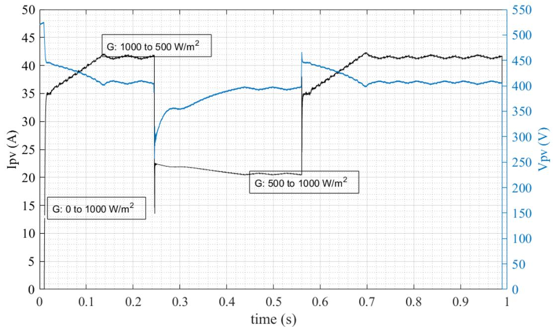
Figure 3.29 Performance of the MPPT controller in presence of rapid irradiance variation at  $T_{pv} = 60 \text{ }^\circ\text{C}$
