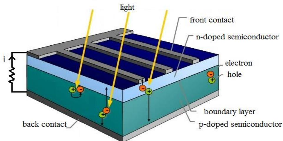
Figure 2.3 Physical structure of a PV cell
