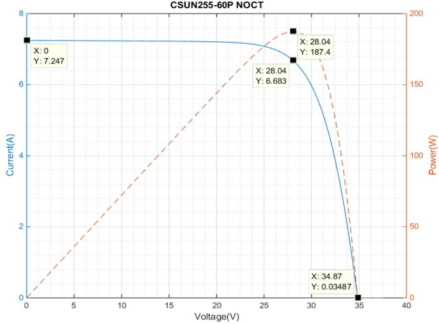
Figure 3.4 P–V and I–V curves of CSUN255-60P at NOCT (800W/m<sup>2</sup> and 45 °C)
