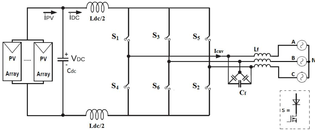
Figure 3.14 Connection diagram of split DC-link inductor
