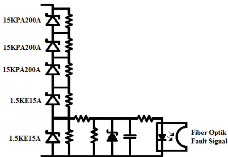
Figure 3.27 Simplified schematic of designed overvoltage protection circuit
