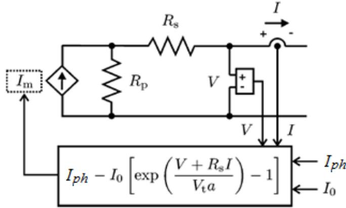
Figure 3.3 PV module equivalent simulation model
