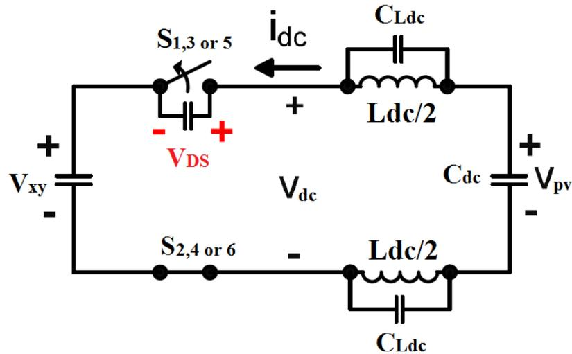
Figure 3.26 Equivalent circuit for DC-link current interruption in a CSI
