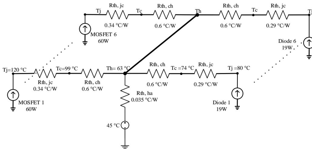
Figure 3.9 Steady-state thermal model
