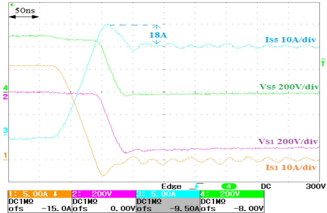
Figure 4.5 Switching waveforms belong to the S1 to S5 commutation event, Ch1: S1 current (orange, 10A/div), Ch2: S1 voltage (pink, 200V/div), Ch3: S5 current (blue, 10A/div), Ch4: S5 voltage (green, 200V/div), time scale 50ns/div, sampling rate 1 GS/s
