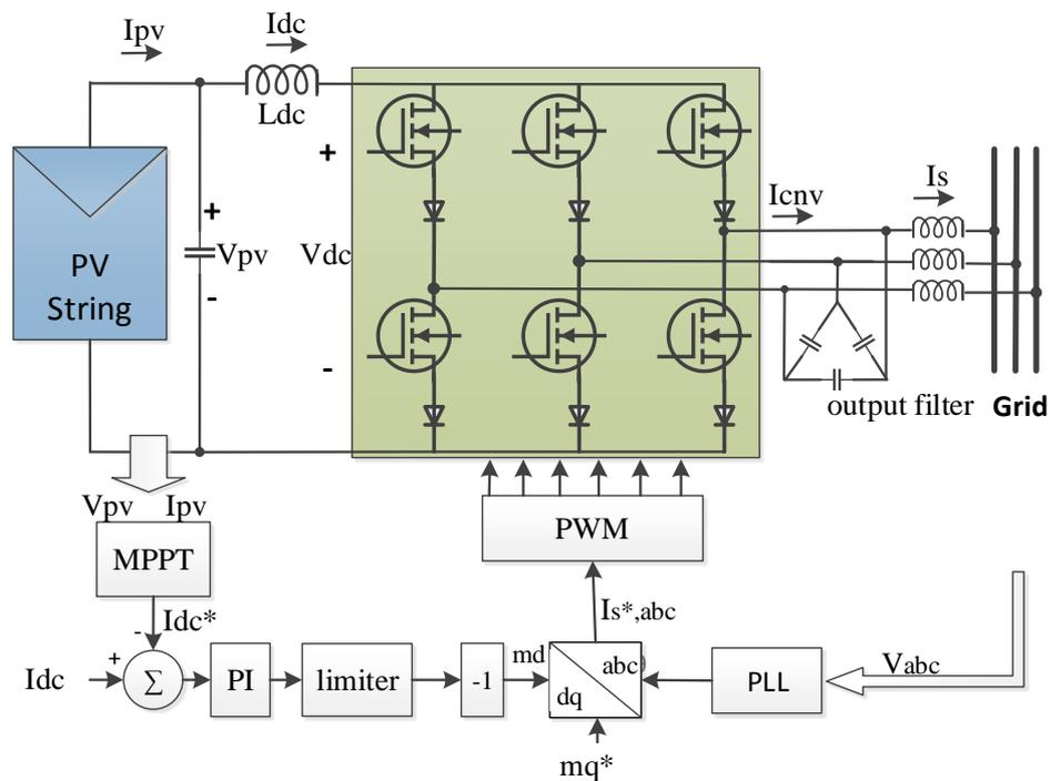
Figure 2.8 Block diagram of power control loop for PV-CSI
