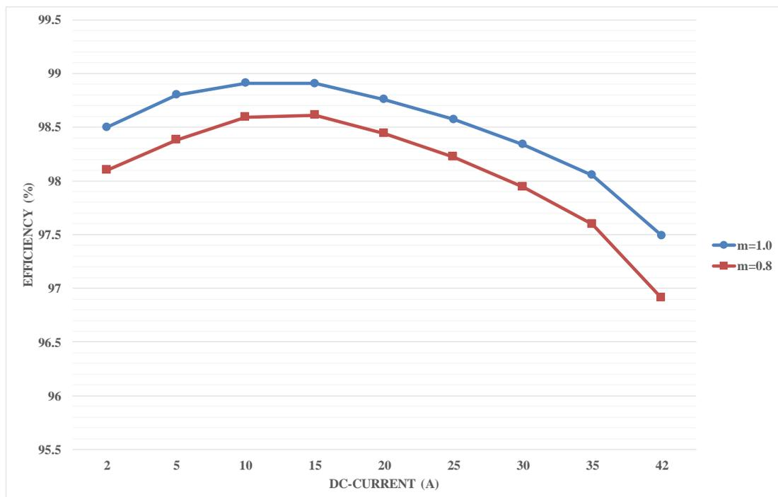
Figure 3.25 Calculated conversion efficiency of the PV-CSI vs DC-link current for  $m=0.8$  and  $m=1.0$
