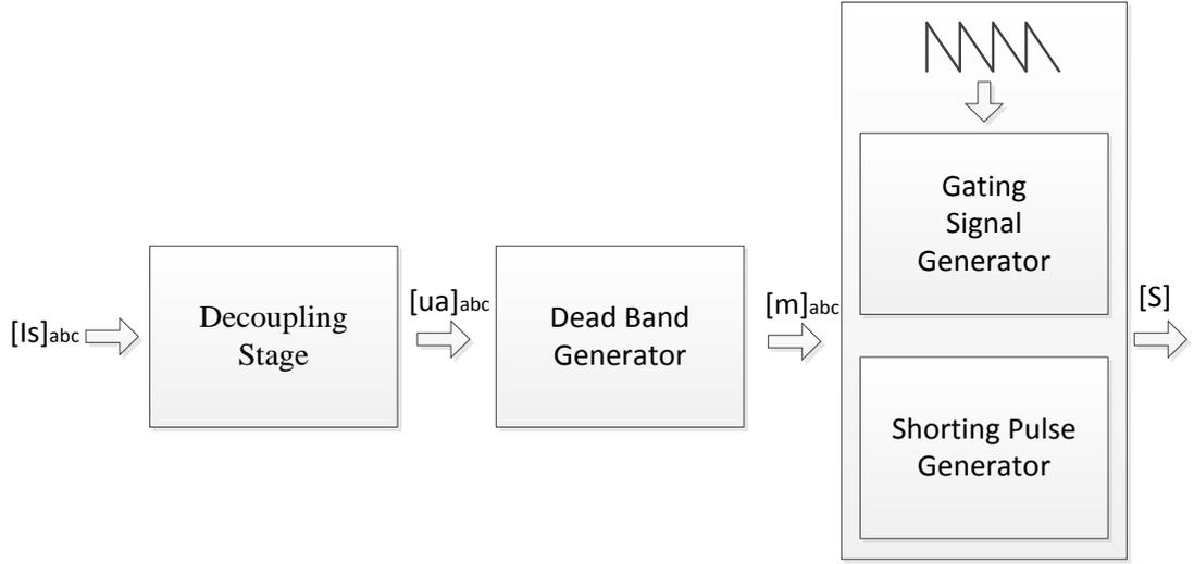
Figure 2.13 Simplified block diagram of the MDSPWM method
