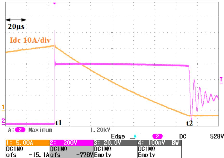
Figure 4.7 Overvoltage protection waveforms in case of an inductor current interruption, inductor current (Ch1:orange, 10A/div), DC-link voltage (Ch:2, pink, 200V/div), time scale 20µs/div
