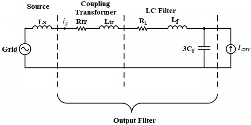
Figure 3.18 Single line diagram of the CSI based grid-connected PV inverter with coupling transformer
