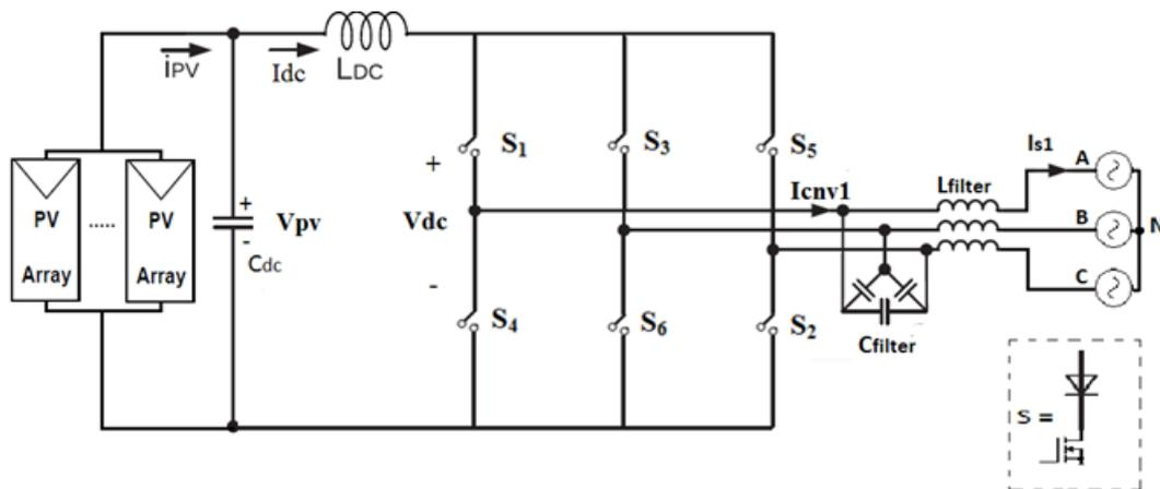
Figure 2.2 Circuit configuration of a three-phase CSI based PV system
