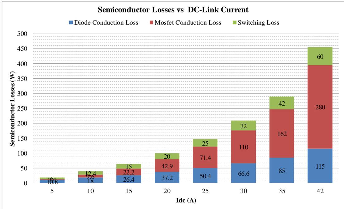
Figure 3.8 Details of semiconductor losses for different DC-link current values
