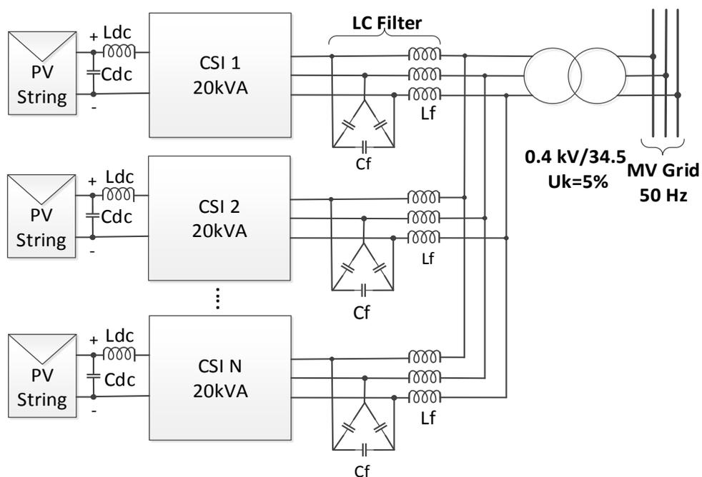
Figure 3.1 Typical large-scale PV power plant based on multi-string inverters
