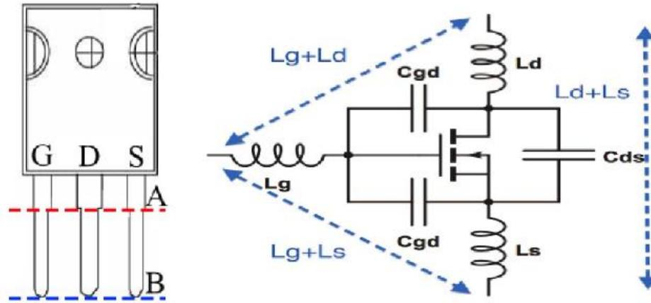
Figure 3.33 Parasitic components on a MOSFET in a TO-247 package
