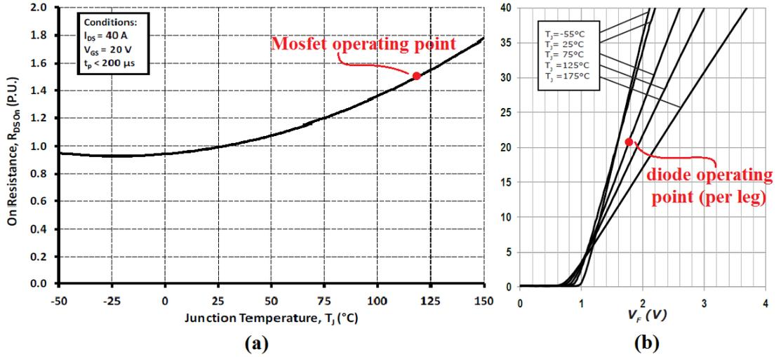
Figure 3.11 ON-state operating points of (a) C2M0040120D, (b) each leg of C4D40120D at rated DC-link current ( $I_{dc}=42$ A)
