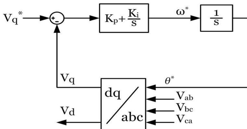
Figure 2.11 Block diagram of the PLL controller
