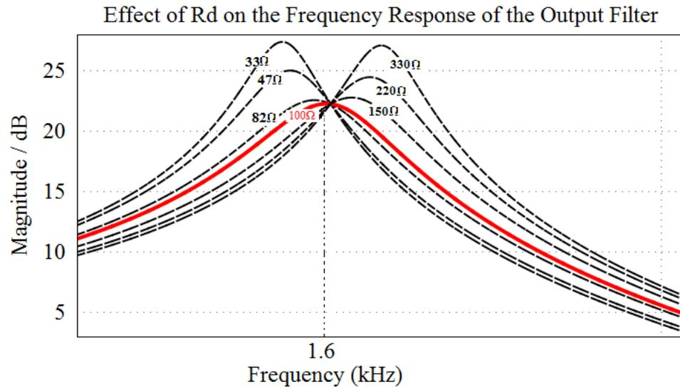
Figure 3.21 Frequency response of output filter for different  $R_d$  values
