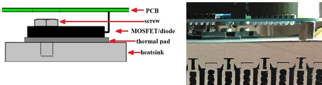
Figure 3.10 Mechanical and electrical connections of the semiconductors
