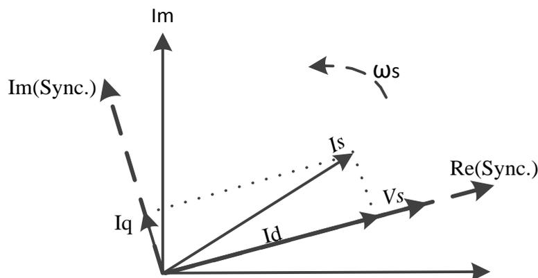
Figure 2.10 Grid Voltage Based Synchronous Reference Frame
