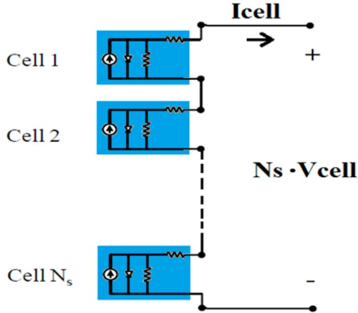
Figure 2.5 Structure of a PV module
