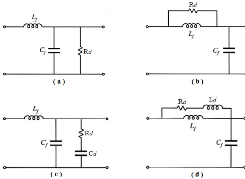
Figure 3.20 Four practical approaches to damping the single-section LC filter: (a)  $R_d$  across  $C_f$ , (b)  $R_d$  across  $L_f$ , (c)  $C_d - R_d$  across  $C_f$ , (d)  $L_d - R_d$  across  $L_f$  [65]
