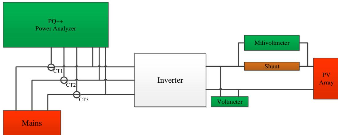
Figure 4.16 Block diagram illustrates the set-up used to measure the efficiency of CSI
