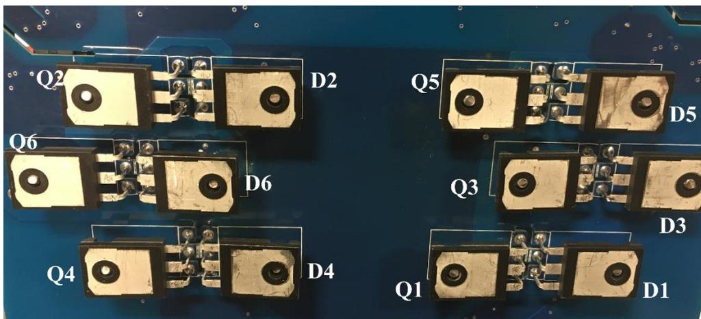
Figure 3.38 Power stage of the PV-CSI prototype (a) top view, (b) bottom view
