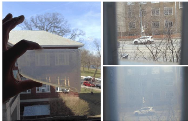
Figure C.10. Monolithic aerogel glazed window (Berardi, 2015).
