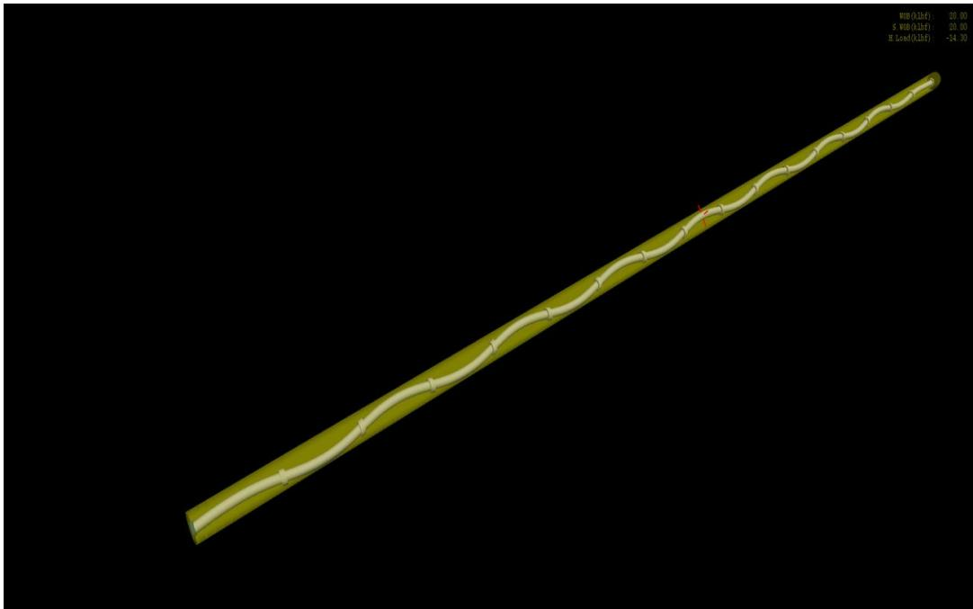
Figure 7-15 3-D View of Drill String under 20 klb WOB
