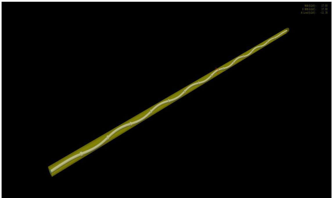
Figure 7-13 3-D View of Drill String under 17 klb WOB
