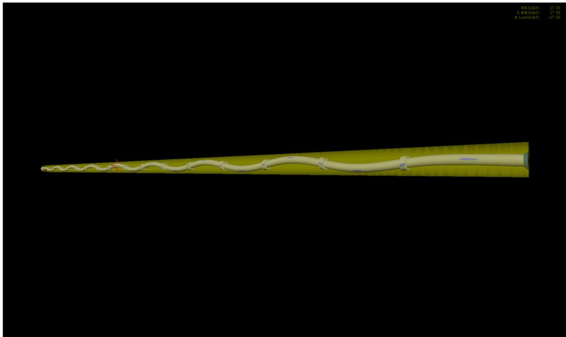
Figure 7-11 3-D View of Drill String under 17.5 *klb* WOB
