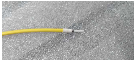
Figure 4.13: Fiber optic cable end, with polished ferrule
