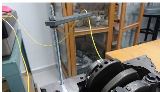
Figure 4.18: Holder used to keep the cables inserted into the bearing caps
