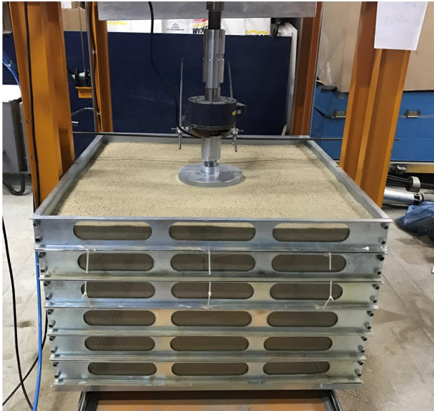
Figure 4.13 Filling of the tank to desired height, placement of loading plate and load cell
