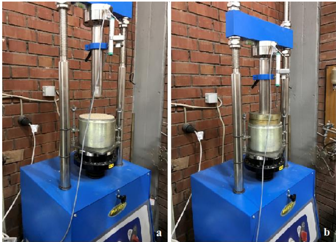
Figure 3.15 California Bearing Ratio (CBR) test
