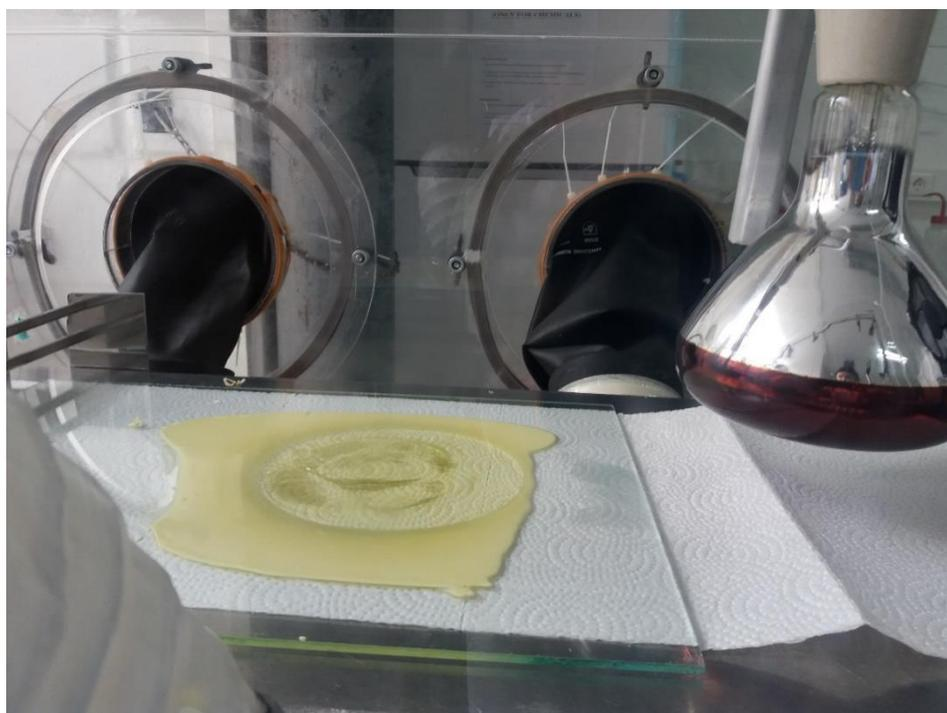
**Figure 3.3** The appearance of the casting PI solution after the light-induced dry phase change, just prior to wet inversion step.
