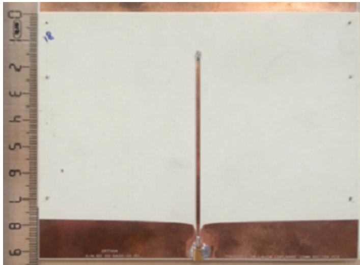
Figure 2.17: Coplanar waveguide to microstrip line transition structure and SMPM connector
