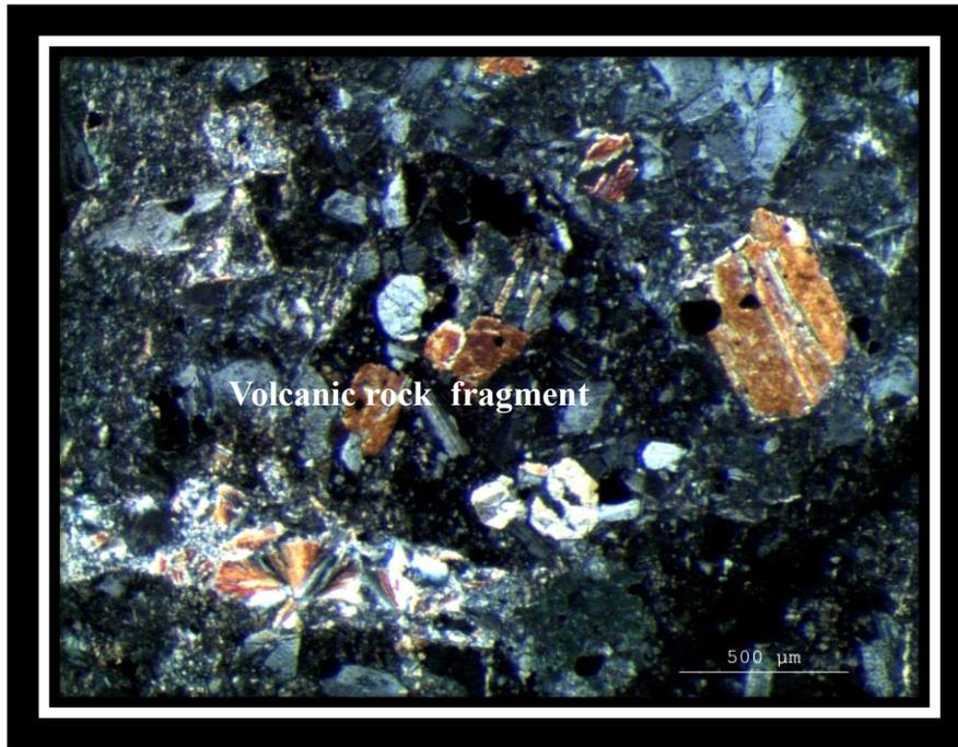
Figure 37. A volcanic rock fragment composed of plagioclase, orthopyroxene and clinopyroxene minerals; as well as Fe-oxide inclusions (XPL).
