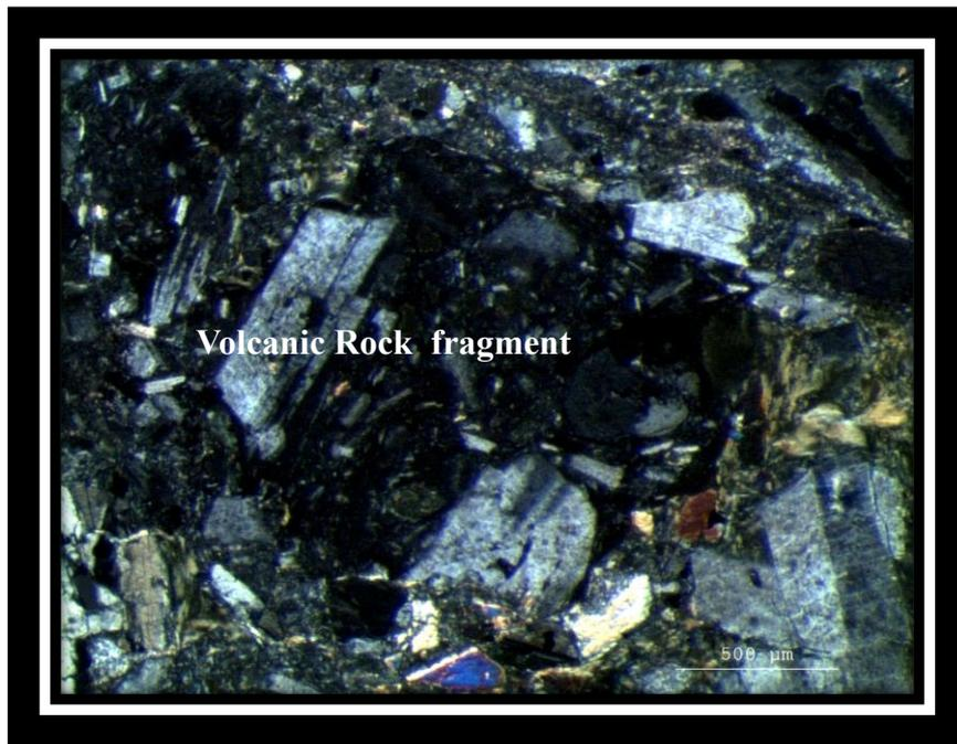
Figure 39. Volcanic rock fragment containing lesser amounts plagioclase minerals as phenocrysts and microphenocrysts and Fe-oxides (XPL).
