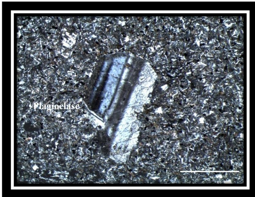
Figure 43. Quenching seen on a plagioclase phenocrystal which partly preserves its crystal boundaries and form.
