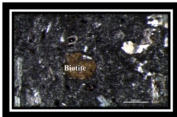
Figure 49. Biotite phenocrystal containing plagioclase mineral and opaque inclusions (XPL).
