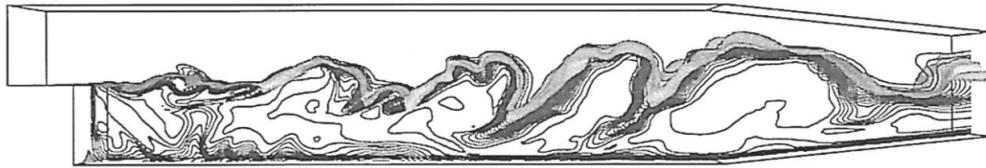
Figure 4.17: Schlieren photograph of the reactive flow [53]
