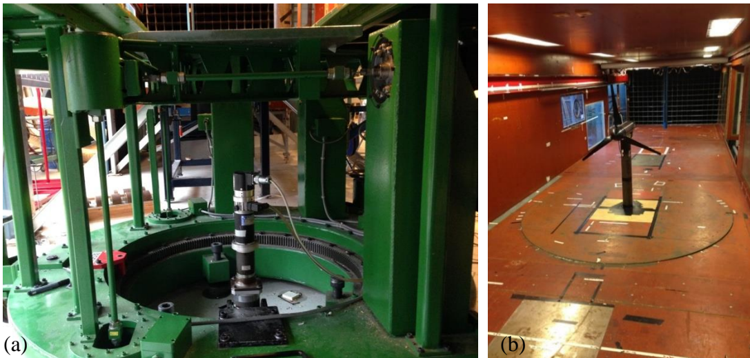
Figure 2-2 (a) Picture of the NTNU closed loop wind tunnel balance system, (b) Picture of the model horizontal axis turbine attached to balance system located inside the NTNU wind tunnel test section
