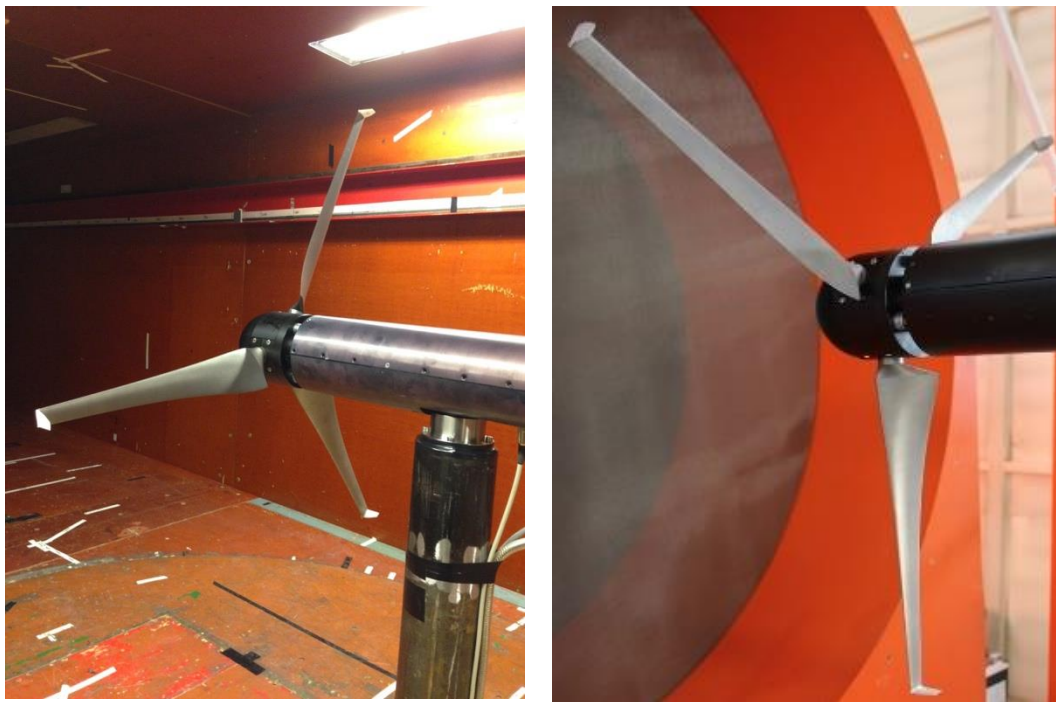
Figure 2-11 Picture of the winglets attached to the blades of the first turbine; (a) Plastic winglets at NTNU closed-loop wind tunnel, (b) Aluminum winglets at METUWIND open jet wind tunnel
