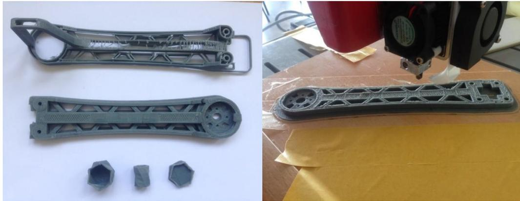
**Figure 4. 12** Photos of two prototypes printed using the custom made 3D printer.
