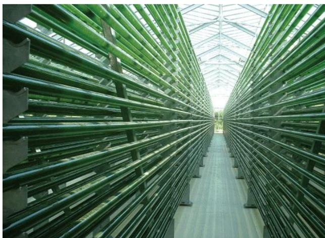
Figure 2-6 An example picture for a horizontal tubular PBR (Iersel et al., 2009)
