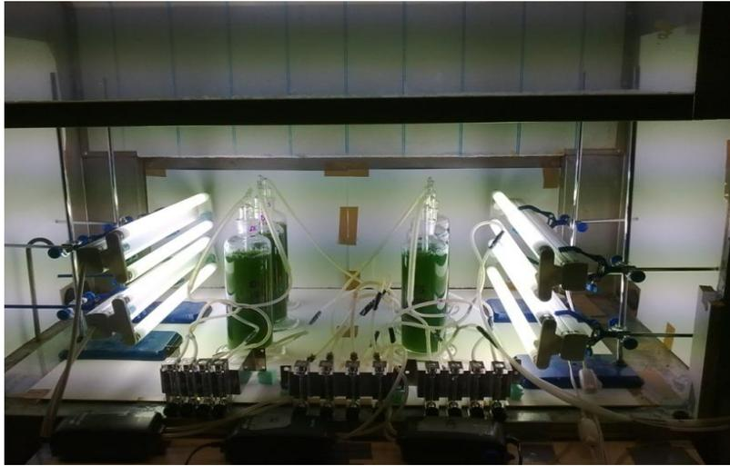
Figure 3-5 A photograph of the set up for the determination of optimum N/P ratio of mixed wastewater
