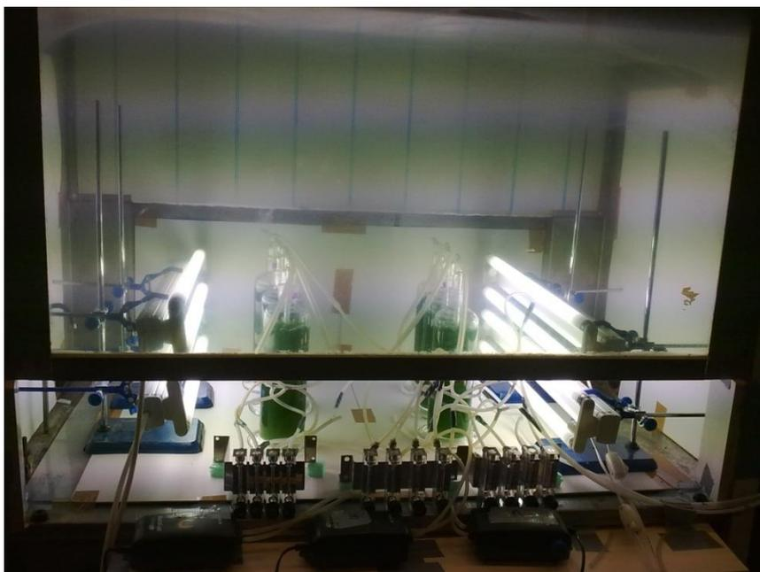
Figure 3-6 A photograph of the set-up run for determination of optimum HRT leading to maximum nutrient removal
