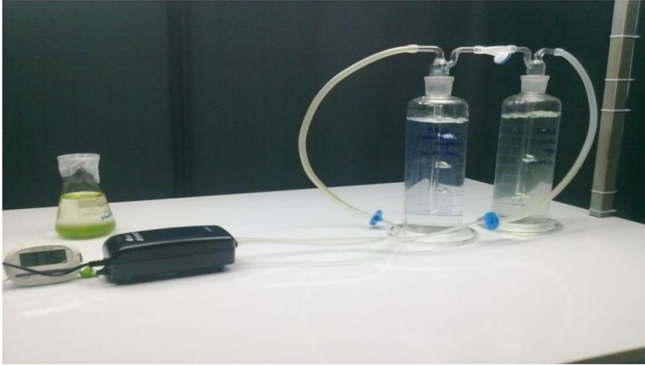
Figure 3-4 The experimental set of cultivating stock *Chlorella Vulgaris* (The reactor on the left is the reactor of axenic *Chlorella vulgaris* culture and the Erlenmeyer flask on the left of the picture is the stock *Chlorella vulgaris* culture).
