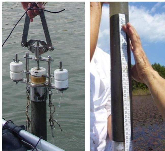
**Figure 1.1** An example of gravity type Kajak Corer.
