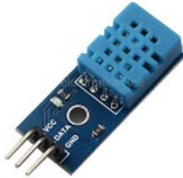
Figure 2.5: Air humidity and temperature sensor
