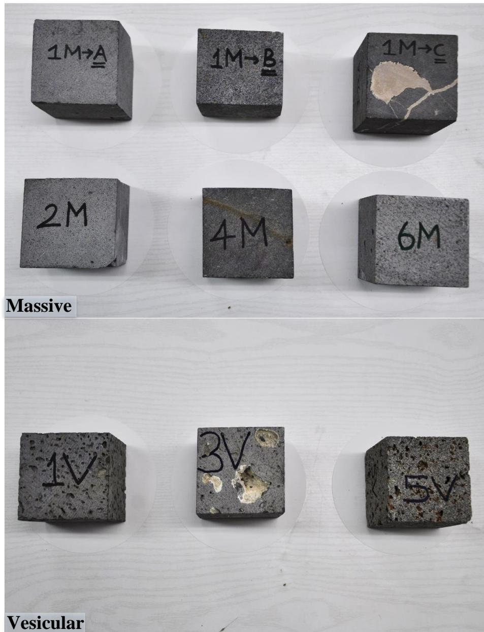
Figure 1.28 The massive and vesicular basalt samples used in the experimental studies
