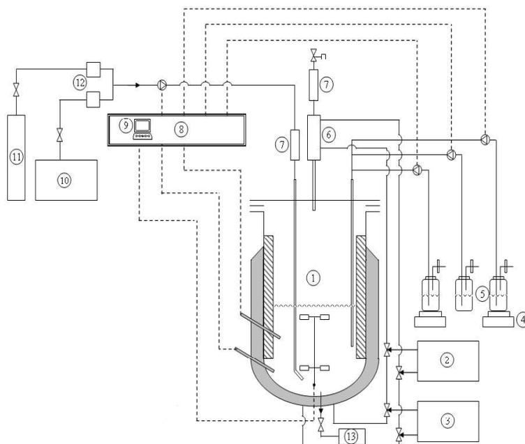
**Figure 3.1:** Illustration of employed 5.0-L bioreactor system: (1) Fermentor, Biostat Cplus 5L (2) Cooler (3) Steam generator (4) balances (5) substrate, antifoam and base resevirs (6) Exhaust cooler (7) Air filters (8) Regulator (9) Biostat Software (10) Air compressor (11) Pure O<sub>2</sub> tank (12) Digital mass flow meters (13) Sampling valve (Çelik, 2008).
